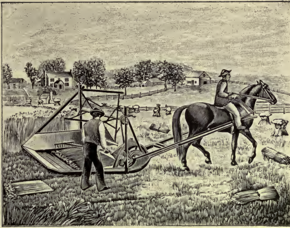
The original McCormick reaper As invented in 1831
