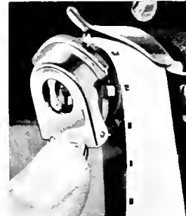
Flip guard against film, and film drops into place and is engaged by sprocket teeth.
