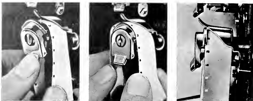
ATTACHMENT GUARDS AGAINST breakage of film on the latest Bell & Howell Filmosounds which feature the sprocket guard pictured and described in these pages. The device also prevents defective films or incorrect splices from jumping the sprocket.
