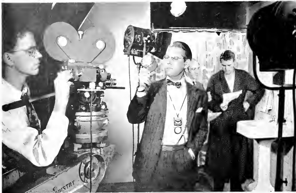
The author takes a reading of color temperature with his Spectra: Films for Industry set.
