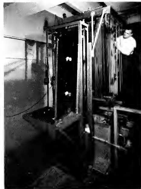
THIS DEVELOPING MACHINE turns a hundred feet a minute—negative or positive—in the processing of black and white film. The precise and efficient Fonda equipment cost $25,000—according to studio notes.
