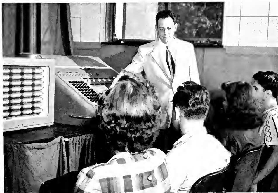
THE COMMUNICATOR IN CLASS USE with Dr. C. R. Carpenter, Penn State professor of psychology in charge. Sloping panel indicates which students answer questions correctly.
