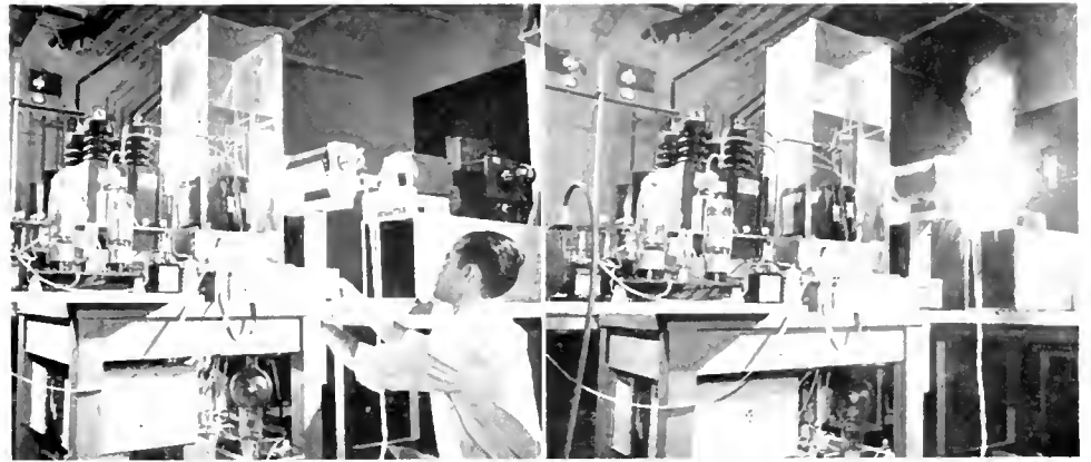
SETTING UP TO SHOOT MOVIES at 100 frames a second recording X-ray exposures of 10 millionths of a second at the Westinghouse lab.
