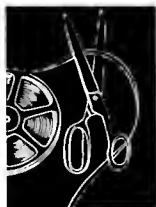
Magnetic tape can be cut, spliced, edited with scissors and Scotch Tape! No tape is ever wasted.
