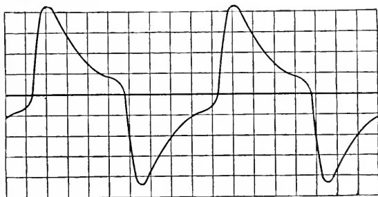
FIG. 2.—Wave without even harmonics.
