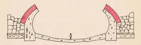
Showing the construction of the floor in the section shown above and also the manner of relining of the sewer as far as the intercepting sewer near C Street.
