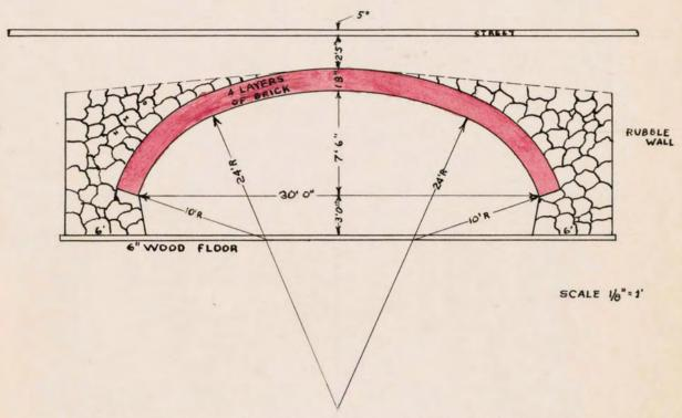
Typical cross-section of the old 30 foot span of Tiber sewer. At Virginia Avenue and South Capitol Street this arch was crossed by the tracks of the Penn. Railroad which subjected it to a considerable live loadand necessitated additional masonry. At this point there was only eight inches of earth separating the railroad tracks from the top of the sewer.
