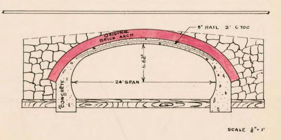
Cross-section of Tiber sewer showing the first section of the relining. This part of the work started at E and North Capitol Streets and extended southwest 107 linear feet. The work was completed on July 26, 1910.
