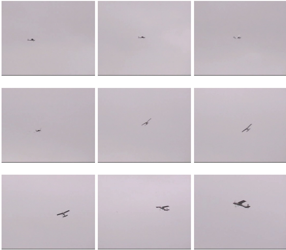
Figure 7.2: A series of still images from video footage showing the transition from pilot control to autonomous control. The frames read from left to right, top to bottom. They are taken at regular intervals every 18 frames which represents approximately 0.71s depicting a controlled turn toward north.
