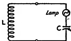
Figure 8A. Absorption Frequency-Meter Circuit
