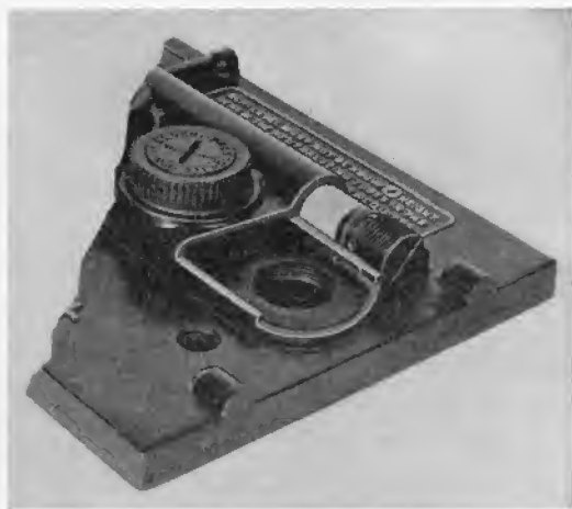
Plate VII. Showing How the Nonspillable Vents Work on a Prestolite Battery
