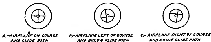
Figure 165. Typical Cross-Pointer Instrument Indications
