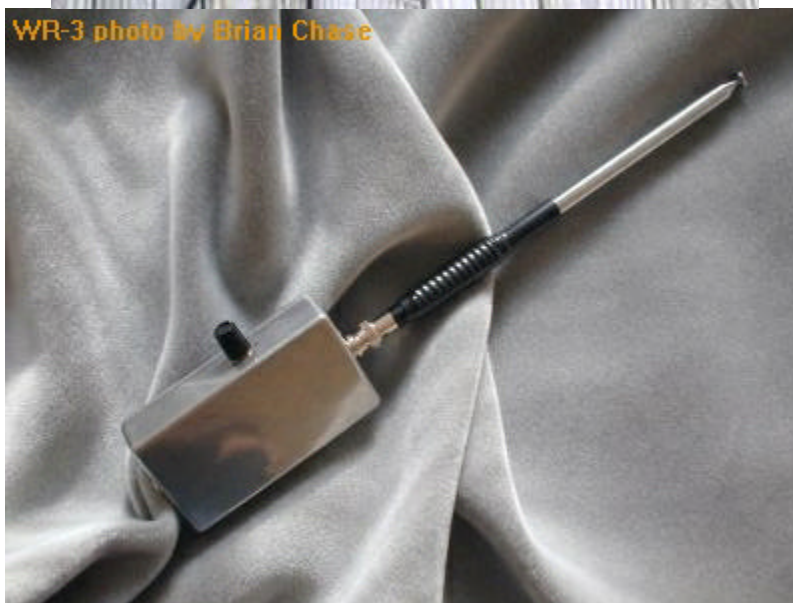
May 2001 photo of the WR-3 shown with Superstick II BNC-base telescoping whip antenna
