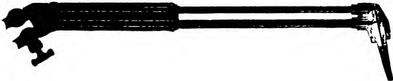
Fig. 8. Section of Pressure-Type Blowpipe
