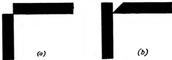
Fig. 61. Corner Welds for Heavy Sheets
