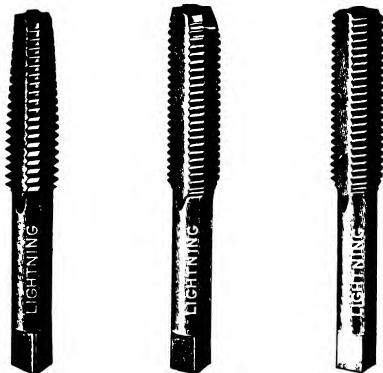
Fig. 33. Types of Hand Taps: Left—Taper Tap; Center—Plug Tap; Right—Bottoming Tap
