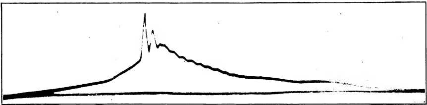
Fig. 57i. Two Cards Indicating Fuel Knock Taken by a Midgley Indicator
