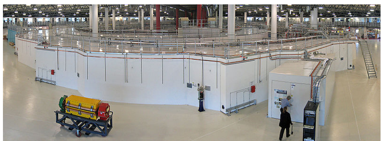
The interior of the Australian Synchrotron facility. Dominating the image is the storage ring, showing the optical diagnostic beamline at front right. In the middle of the storage ring is the booster synchrotron and linac
