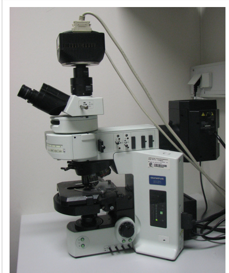
A fluorescent microscope (Olympus BX61), coupled with a digital camera.
