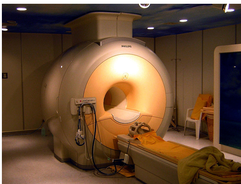
Advanced 4.7 T clinical diagnostics and biomedical research NMR Imaging instrument.
