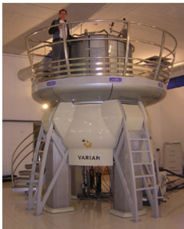
A 900MHz NMR instrument with a 21.2 T magnet at HWB-NMR, Birmingham, UK, being loaded with a sample.
