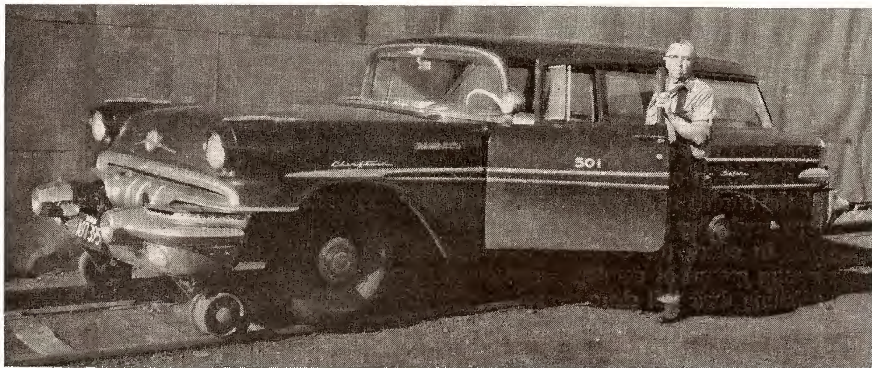
Roger F. Otis, repairman for the Work Equipment Shops, enters the Engineering Department's high rail inspection car. The car is a Pontiac, nine passenger station wagon, with a special Fairmont pneumatic attachment to lower wheels for use on track, and to raise them when the car moves from track to highway use. The Work Equipment Shop attached wire brushes back of the rail wheels to provide contact for setting track signals as the car moves on track.
