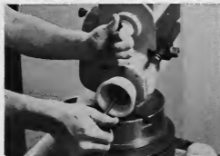
Figure M16A MOUNTING THE GRINDING WHEEL AND COLLET ASSEMBLY
