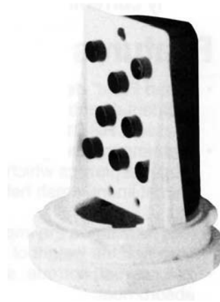
Figure 3-45: "Dead-Front" Test Station
