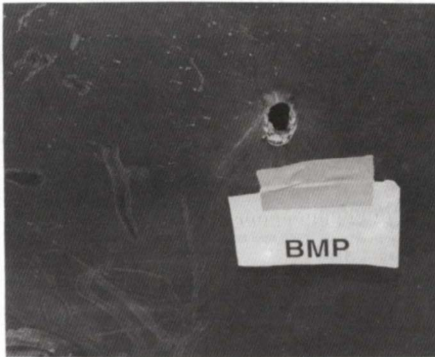
DU kinetic energy impact entry hole with spalling on Soviet BMP.
