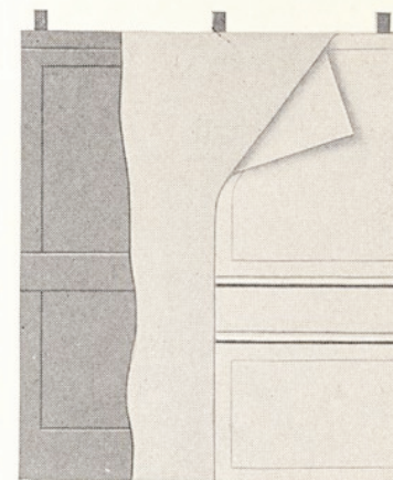
Cop-R-Loy steel stretcher leveled steel, then ample felt to eliminate rumbles over waterproof three-ply veneer are the basic elements in E-B Panel Bodies.
