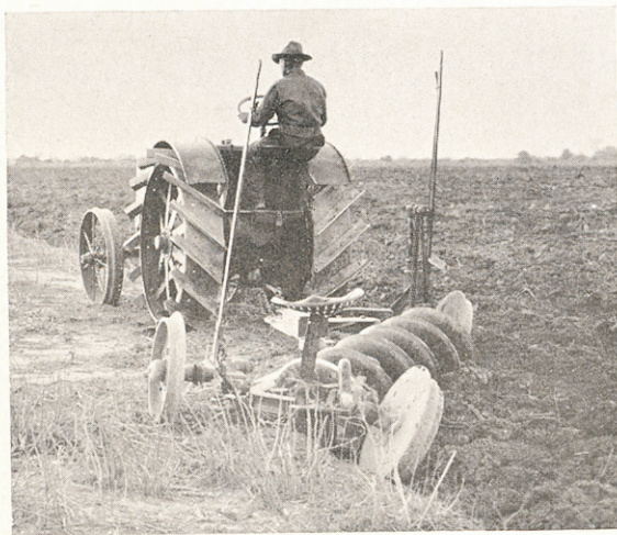
E-B 12-20 Model AA pulls from four to six discs in the hardest kind of soil
