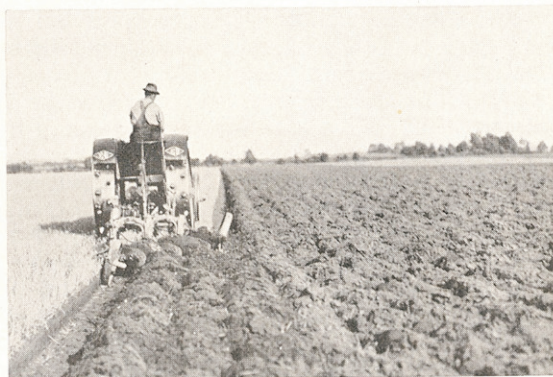
The E-B 12-20 Model AA is a three plow tractor
