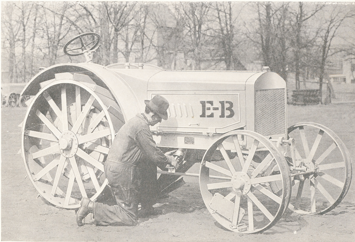
View showing one of the two hand hole plates removed from motor base, note the easy working position of operator
