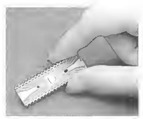
frammond engineering leadership is reflected in the exclusive LSI (Large Scale Integrated) multiplex synthesis circuitry for the Colonnade. These custom LSI circuits contain up to 8,000 separale electronics devices in each tiny (about 1/4" square) chip. The result is outstanding performance and musical integrity with unmatched reliability.
