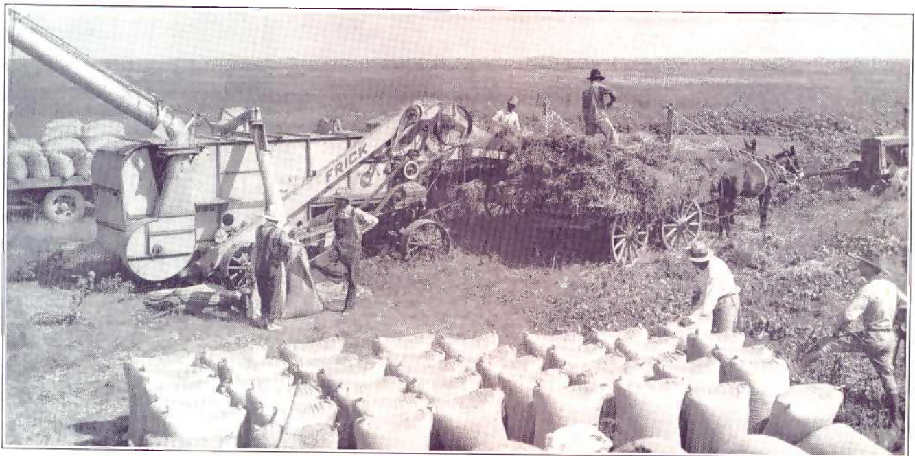
In the 1930's Frick steel threshers were adapted to handling rice, and are now used for this purpose throughout the globe. This machine is at work in the flat Louisiana rice fields: note large sacks of grain.
