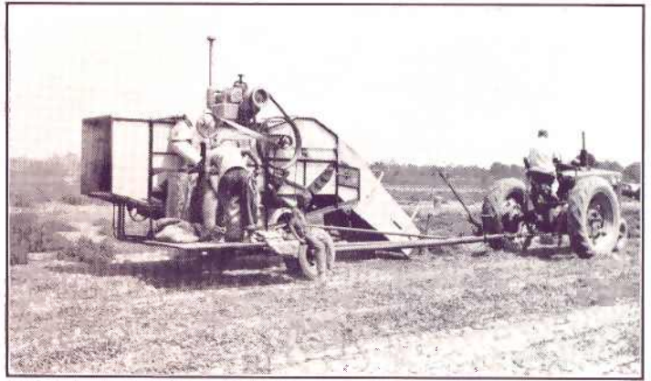
The peanut combine, introduced in recent years, saves labor in areas where the nuts can be harvested in windrows.
