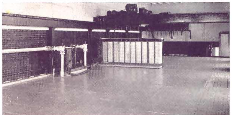
Average-sized ice tank, using the patented F-P system and Frick group lift. Electric Ice Manufacturing Co., Richmond, Va.
