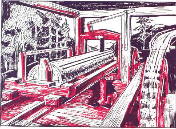
A sawmill of this "up-and-down" type, driven by water power, was operated by Abraham Frick about 115 years ago. Boards cut by this method were split off the log near the end; they can still be identified in some old barns.
