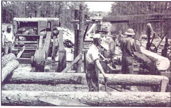
This sawmill, kept humming by a pair of engines, cut as much lumber as two mills, operated by separate crews, had formerly done.
