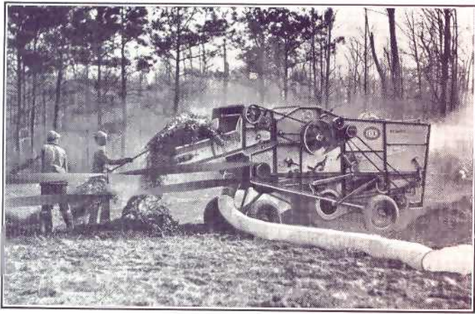
Frick steel peanut pickers, introduced in 1938, are still going strong. Cleaner, faster, and more durable, they enjoy a natural preference.
