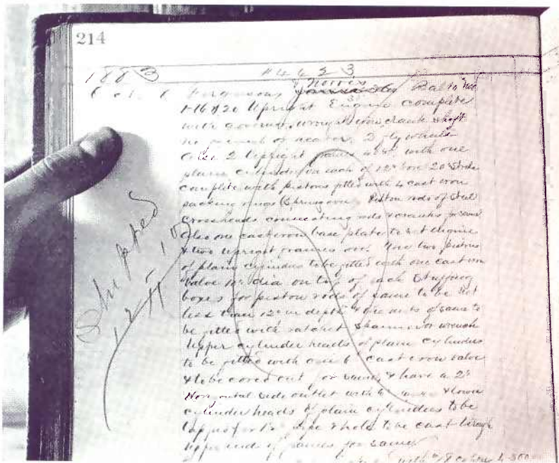
The first complete Frick refrigerating machine, built in 1883, had two ammonia cylinders of 12-in. dia. by 18-in. stroke, with a steam cylinder between them. It ran at 50 to 55 r.p.m., and developed 25 tons of refrigeration. As shown at left, the order can still be seen on Frick Company's books.
