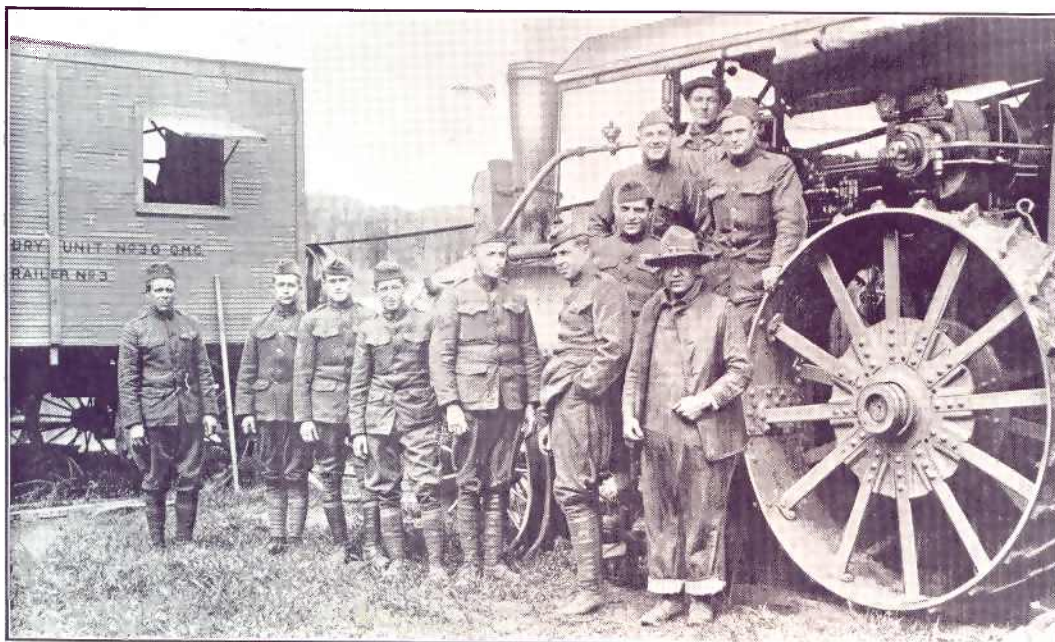
Left: Traction engine furnishing both power and steam to an Army Laundry Unit, somewhere in France, 1917-1918.
