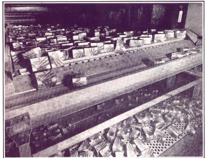
Quick-freezing tunnel, 120 ft. long, hardening 180 pint packages of ice cream a minute; temperature, 50 to 55 deg. F. below zero. Hershey Creamery Co., Harrisburg, Penna.
