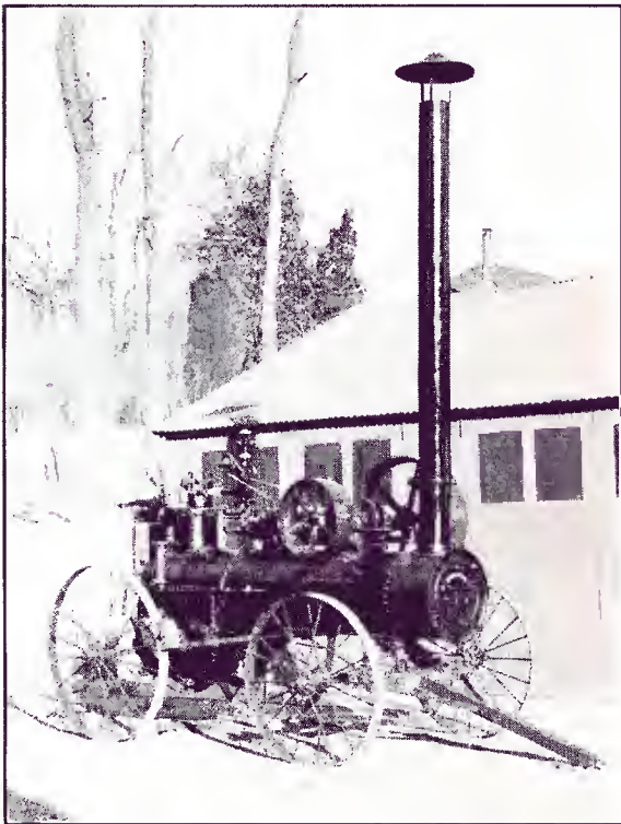
Moving a 30-ton house half a mile with a Frick traction engine. These machines crushed stone, built roads, pumped water, operated mills, and did many other kinds of belt and drawbar work.
