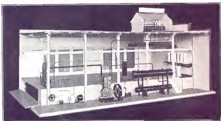
Model of a dual-pressure ice plant, in which the water and liquid ammonia are precooled at high suction pressure, with about 10 per cent extra efficiency.
