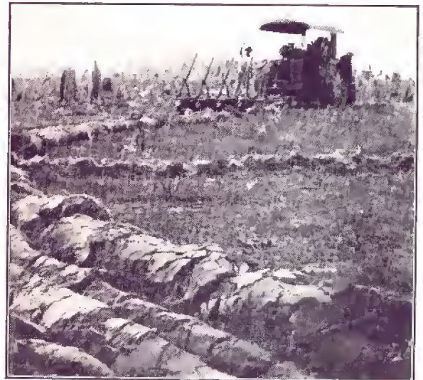
Heavy traction engine demonstrating its plowing ability in "new-ground." These big rigs were usually worked by two men.
