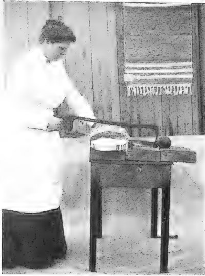
No. 1—Cutting material with a weighted knife, which saves hours of tedious cutting with scissors, or tearing.
