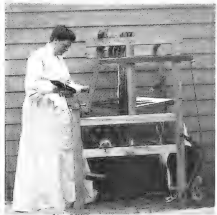
No. 2—Making experiments in weaving border designs in a narrow loom. In changing the color of the warp the brown threads have been tied to the white which was already on the loom. The lay-to is brought sharply forward to make the warp firm.
