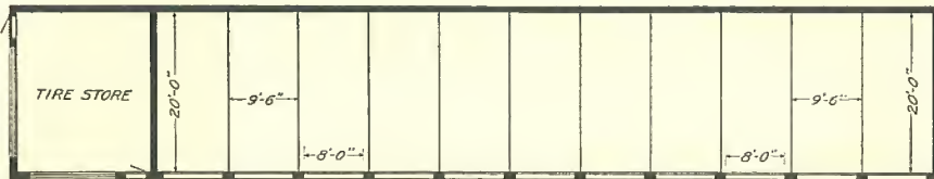
A garage with eleven private, steam-heated stalls. Doors hung with No. 806 Garage Door Sets. (Equipment, pages 18 to 21.)
