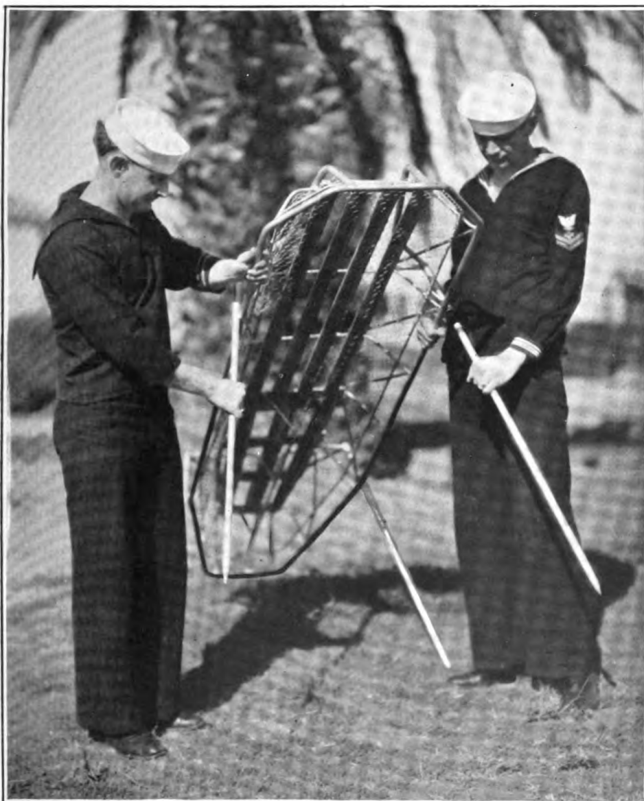
INSERTING THE SUPPORTS USED TO CONVERT STRETCHER INTO A FIELD DRESSING TABLE.
