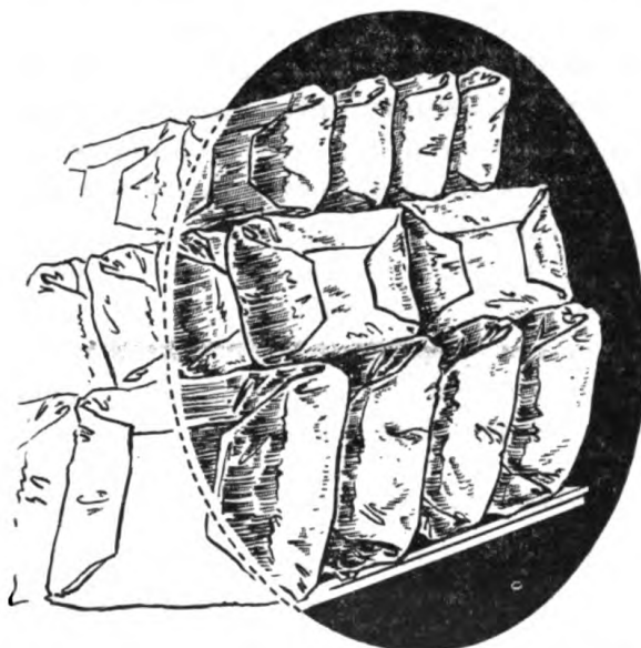
FIGURE 12.—Illustrates correct arrangement of packs in a large sterilizer not equipped with shelving.
