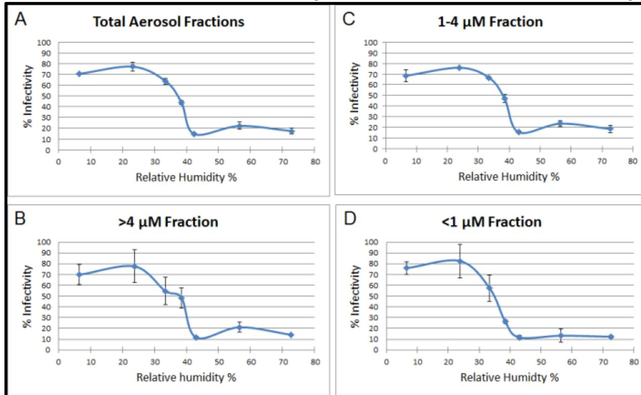
Infectious virus was coughed into the simulated exam room. The relative humidity in the simulated exam room was varied over 7-73% at 20°C.
