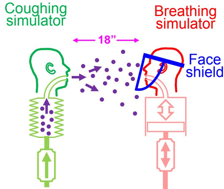
Coughed broader size range of influenza particles (0.1  $\mu\text{m}$  to 100  $\mu\text{m}$ ).
