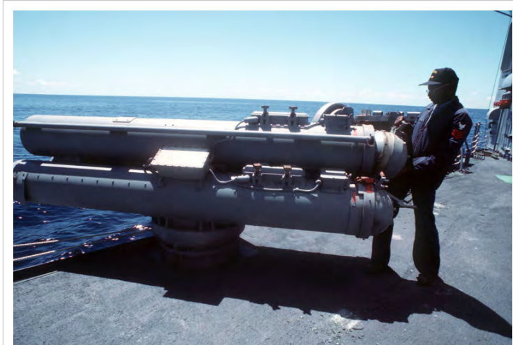
A crewman closes the breach of a Mark 32 12.75-inch torpedo launcher aboard the → Oliver Hazard Perry -class guided missile frigate → USS Curtiss (FFG-38) during anti-submarine warfare operations off the coast of Southern California
