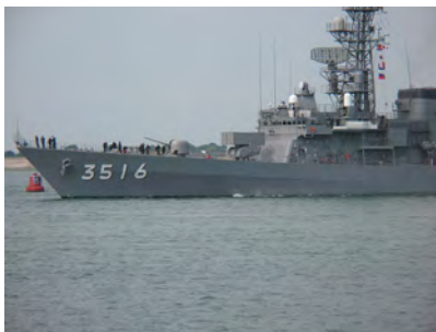
The OTO-Melara 76mm mounting is seen in this photograph of the Japanese Asagiri class destroyer Asagiri , formerly DD 156, renumbered TV 3516, seen here on 28 July 2008 departing from Portsmouth Naval Base, UK.
