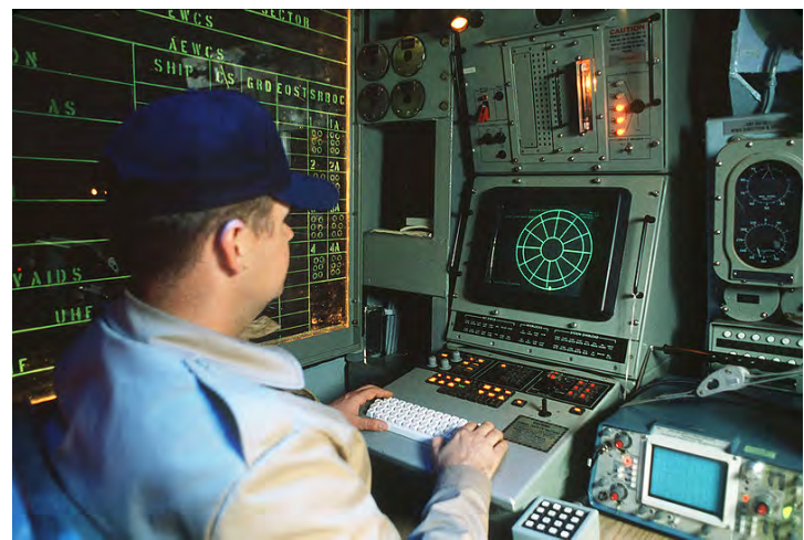
AN/SLQ-32 console aboard USS Iowa (BB-61).
