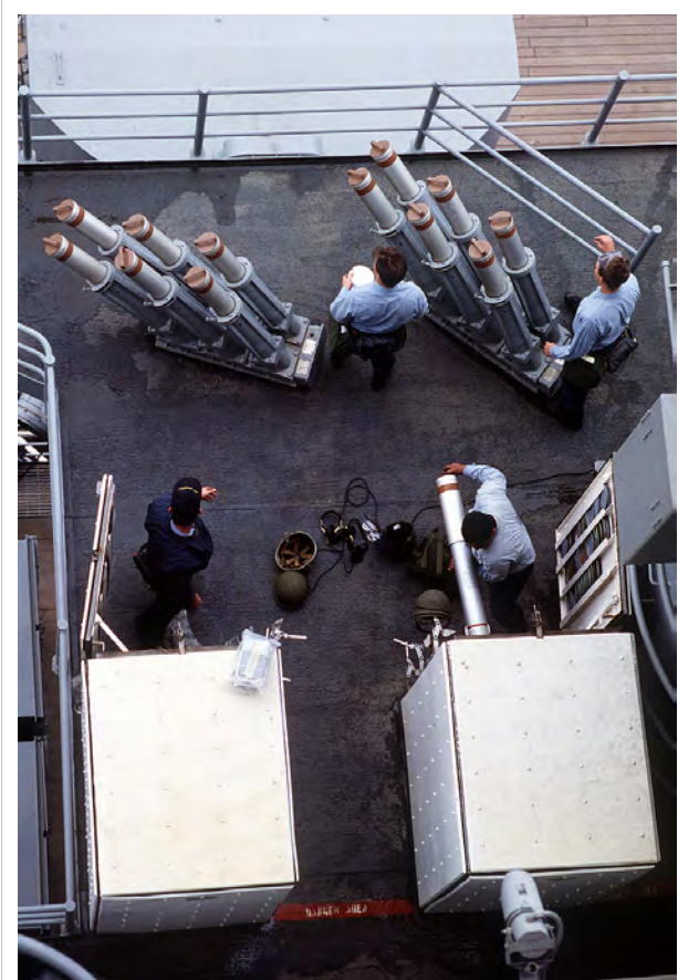
Two Mark 36 Mod 7 Super Rapid Bloom Off-board Chaff (SRBOC) system launchers aboard the battleship USS Wisconsin (BB-64) during Operation Desert Storm.
