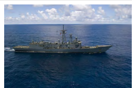
→ USS Rodney M. Davis (FFG-60) after the removal of her foredeck → Mk 13 missile launcher.
