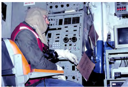
A sailor sits in front of a CIWS Local Control Panel (LCP) during a general quarters drill.
