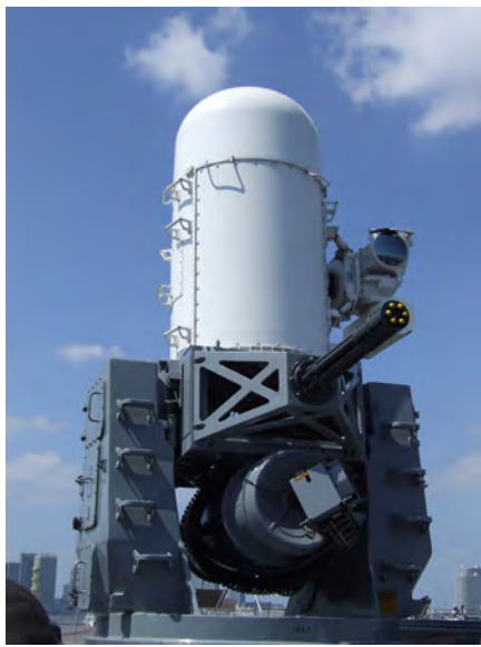
Block 1B Phalanx, displaying the FLIR and improved barrel
