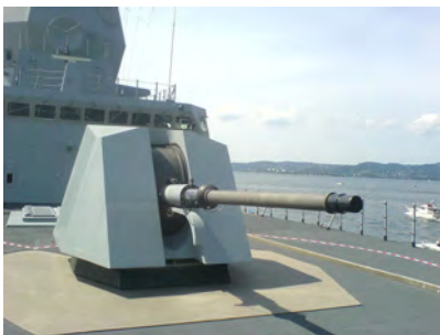
On the Norwegian Fridtjof Nansen -class frigates, the Oto Melara is equipped with a stealth cupola to reduce radar cross section/
