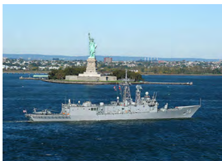
Simpson arriving in New York Harbor, October 2004 prior to removal of Mk 13 launcher, but after removal of the STIR missile guidance radar.
