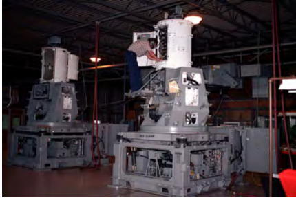
A technician checks over the RADAR transmitter and microwave assemblies of a Phalanx CIWS, most likely a Block 0. The search radar can be seen at the top with the vertical, orange-peel shaped, tracking radar below it.
