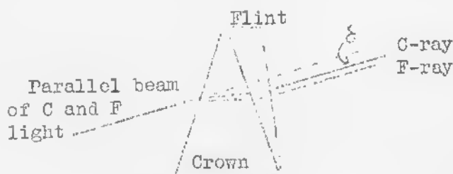
Fig. 18. A combination achromatized for C- and F-light.
