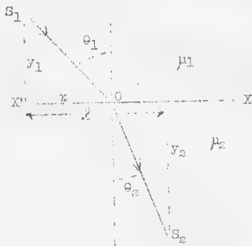
Fig. 6. The Fermat principle applied to refraction at a plane surface.
