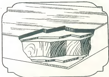
Armstrong inlaid linoleum, jasper finish, mounted on heavy plywood top prevents warping and insures long life of service.
