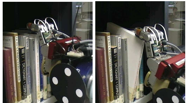
Fig. 5. The robot grasping the book by means of sensor-based continuous estimation of hand-to-object relative pose.
