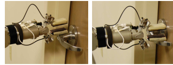
Fig. 5. Finding the tip of the door handle that can be moved down or declaring the handle to be locked. Left image: Rigid tip, Right image: moveable tip.
