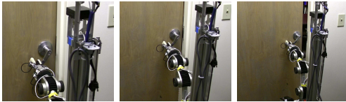
Fig. 7. Left to right: Robot twists the door handle until the end. Robot pushes the door and estimates the doorway. Robot pushes the door so that the handle can be released.
