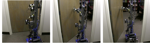
Fig. 8. Left image: Positioning itself to prevent collision with the wall. Right two images: Traversing through the doorway while pushing the door open.
