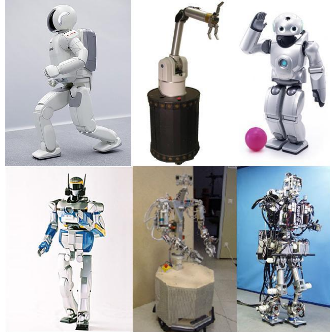
Fig. 1. Examples of Mobile Manipulators. Top: Asimo (Honda), UMan (UMass Amherst), QRIO (Sony) Bottom: HRP-3 (Kawada Industries), AR-MAR (University of Karlsruhe), WABIAN RIII (Waseda University Tokyo)
