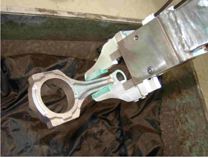
Fig. 1. Standard industrial two-fingered gripper using a nominal grasp to grip a con-rod [14].
