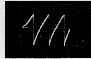
Figure 43—Horizontal Oscil- lator Output (60 Volts, P to P) (Junction of C135 and C163)
