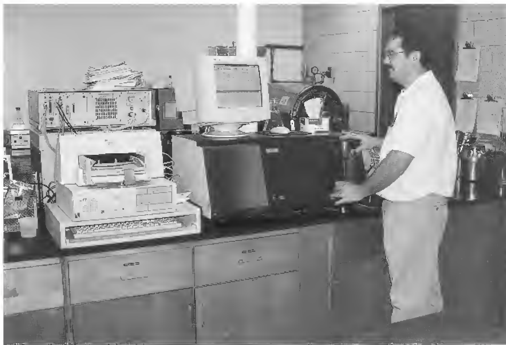
Figure 4 Automated method of fat and total solids measurement for milk and milk products. (Photograph courtesy of Mayfield Dairies and Dean Foods Company, Athens, TN.)
