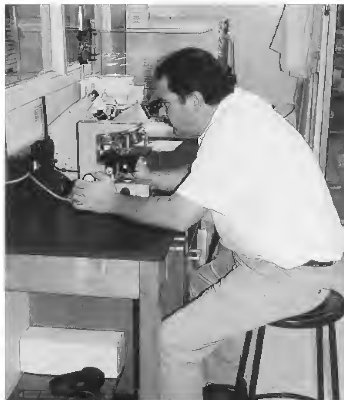
Figure 6 QA technician doing DMC on incoming raw milk. (Photograph courtesy of Mayfield Dairies and Dean Foods Company, Athens, TN.)
