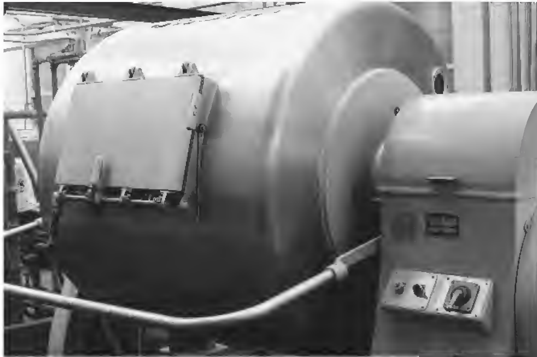
Figure 10 A batch churn with controls. A few batch churns continue to operate in the United States.
