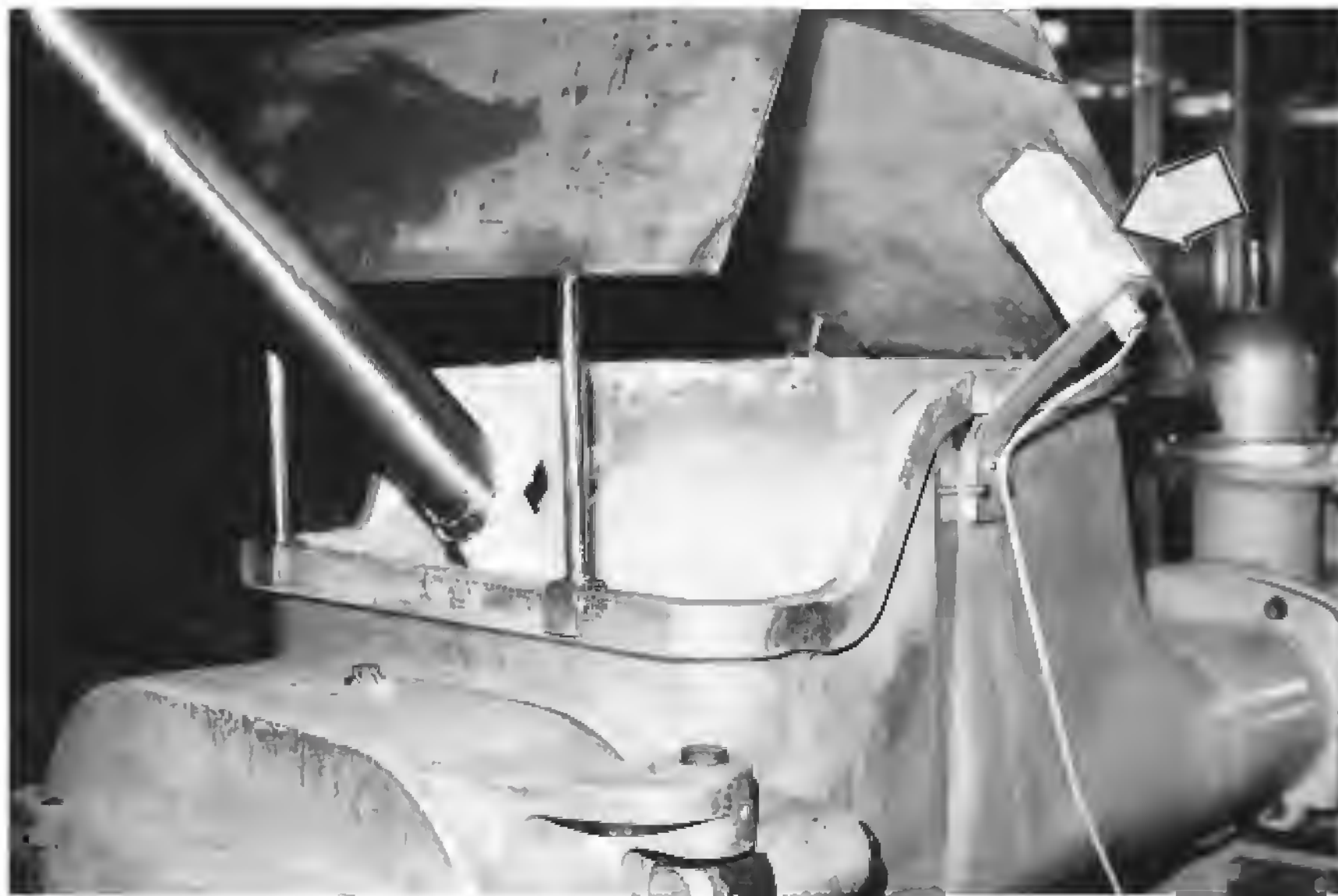
Figure 7 Infrared light sensor ( arrow ) monitors level of butter in hopper and signals computer which controls off/on of delivery pump and an air-operated valve.
