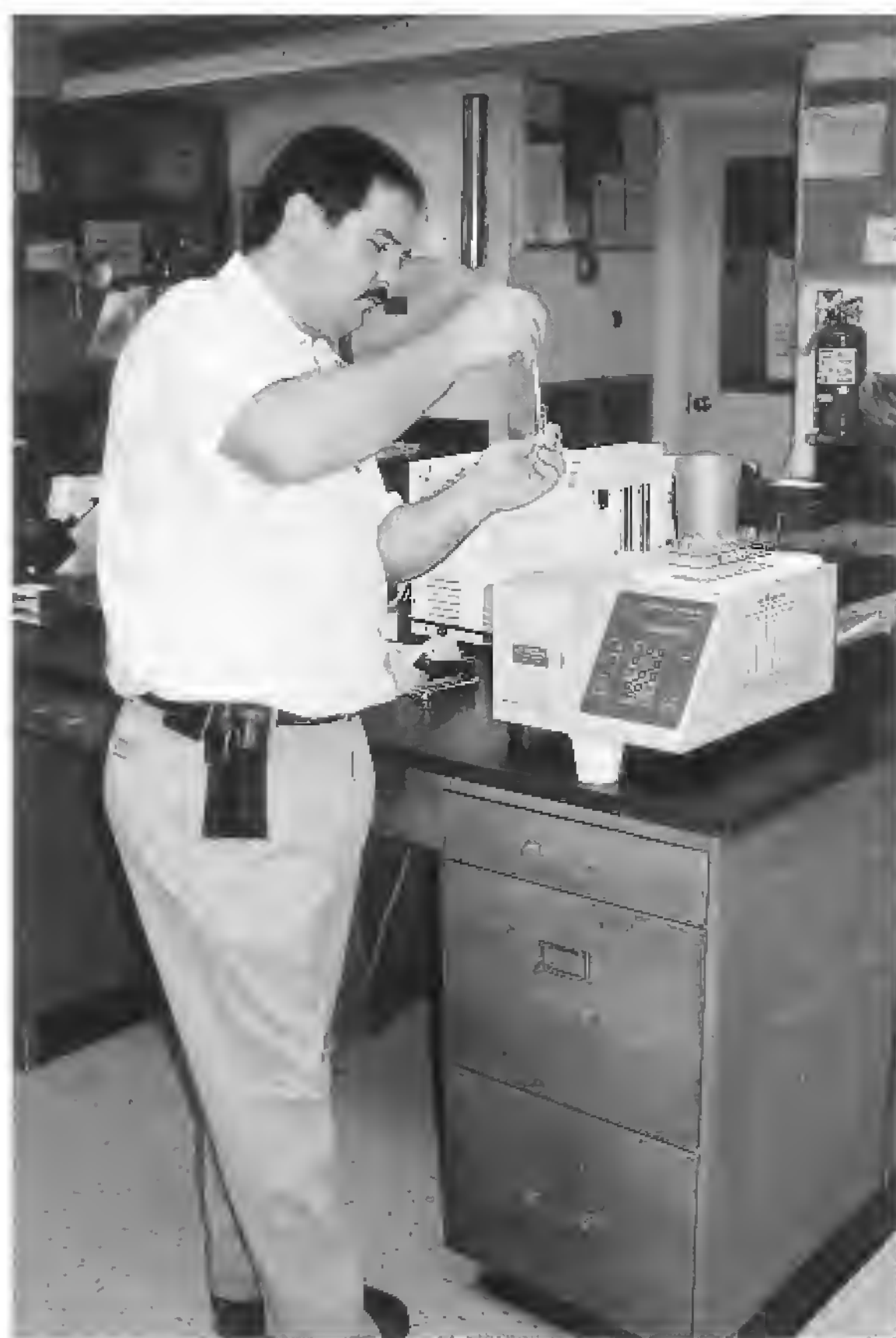
Figure 2 QA technician measuring freezing point of milk to check for added water. (Photograph courtesy of Mayfield Dairies and Dean Foods Company, Athens, TN.)
