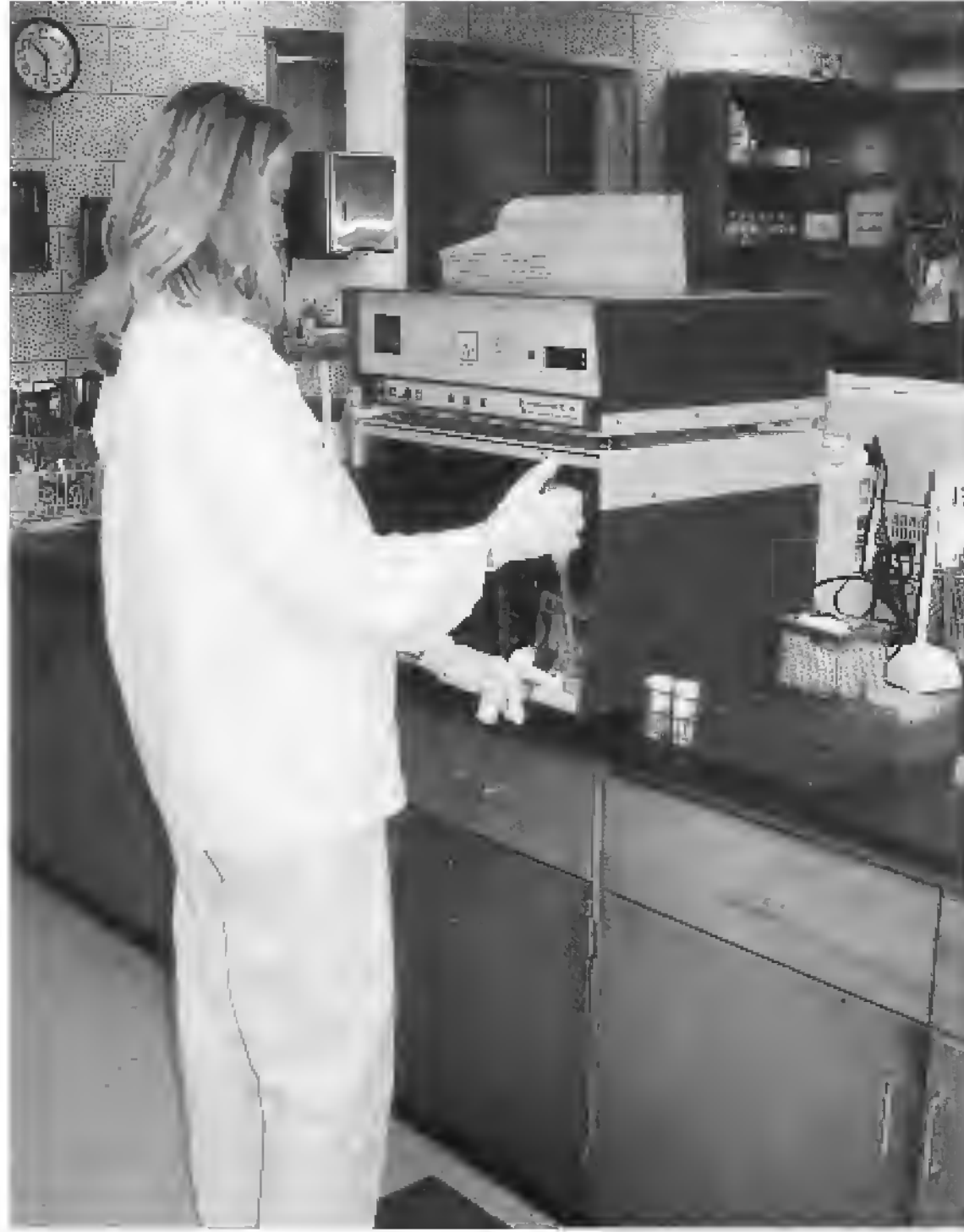
Figure 1 QA technician determining estimate of somatic cell numbers in raw milk using the latest instrument. (Photograph courtesy of Mayfield Dairies and Dean Foods Company, Athens, TN.)
