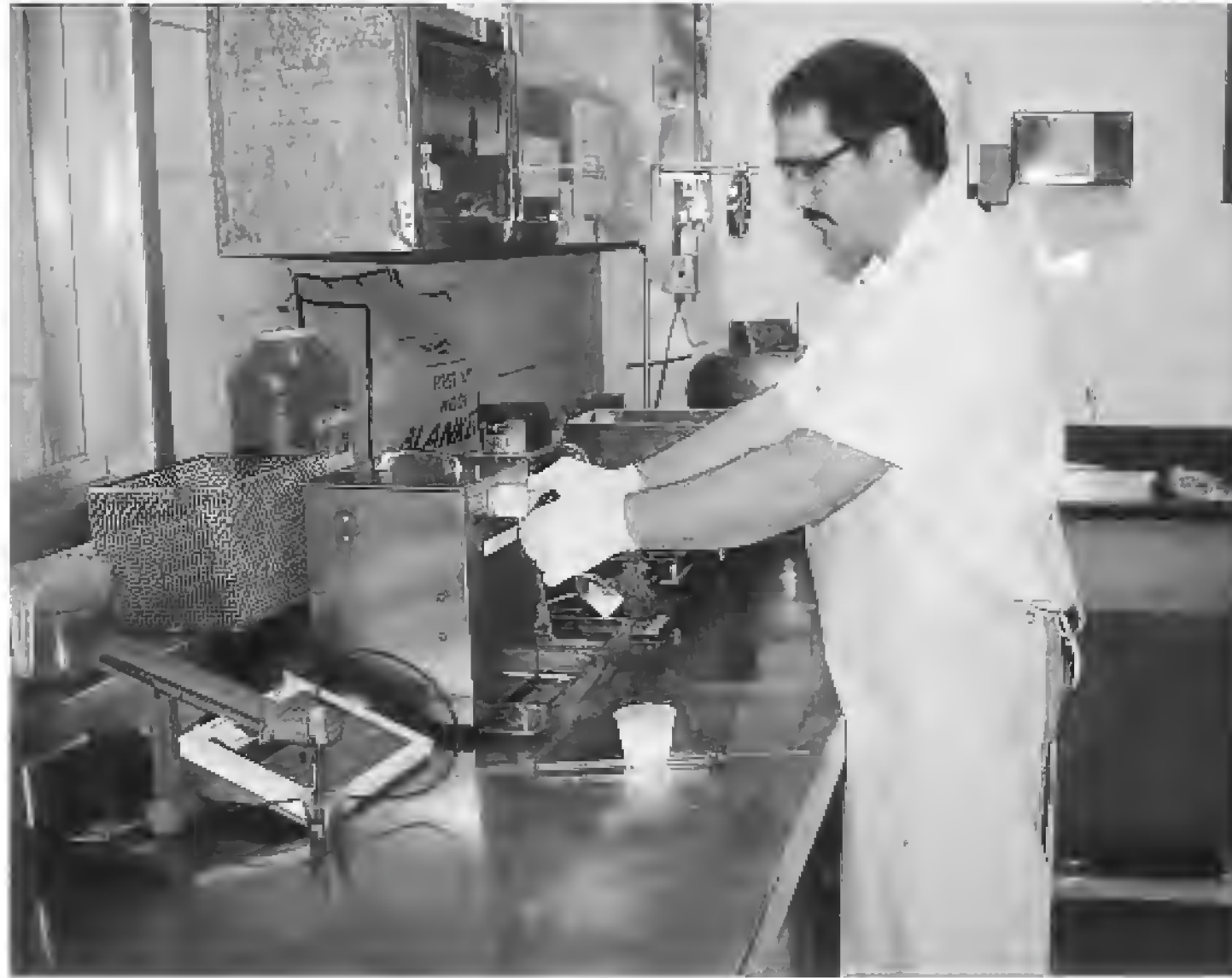
Figure 3 QA technician measuring fat content of raw milk using Babcock method—note safety equipment required (apron, gloves, goggles). (Photograph courtesy of Mayfield Dairies and Dean Foods Company, Athens, TN.)
