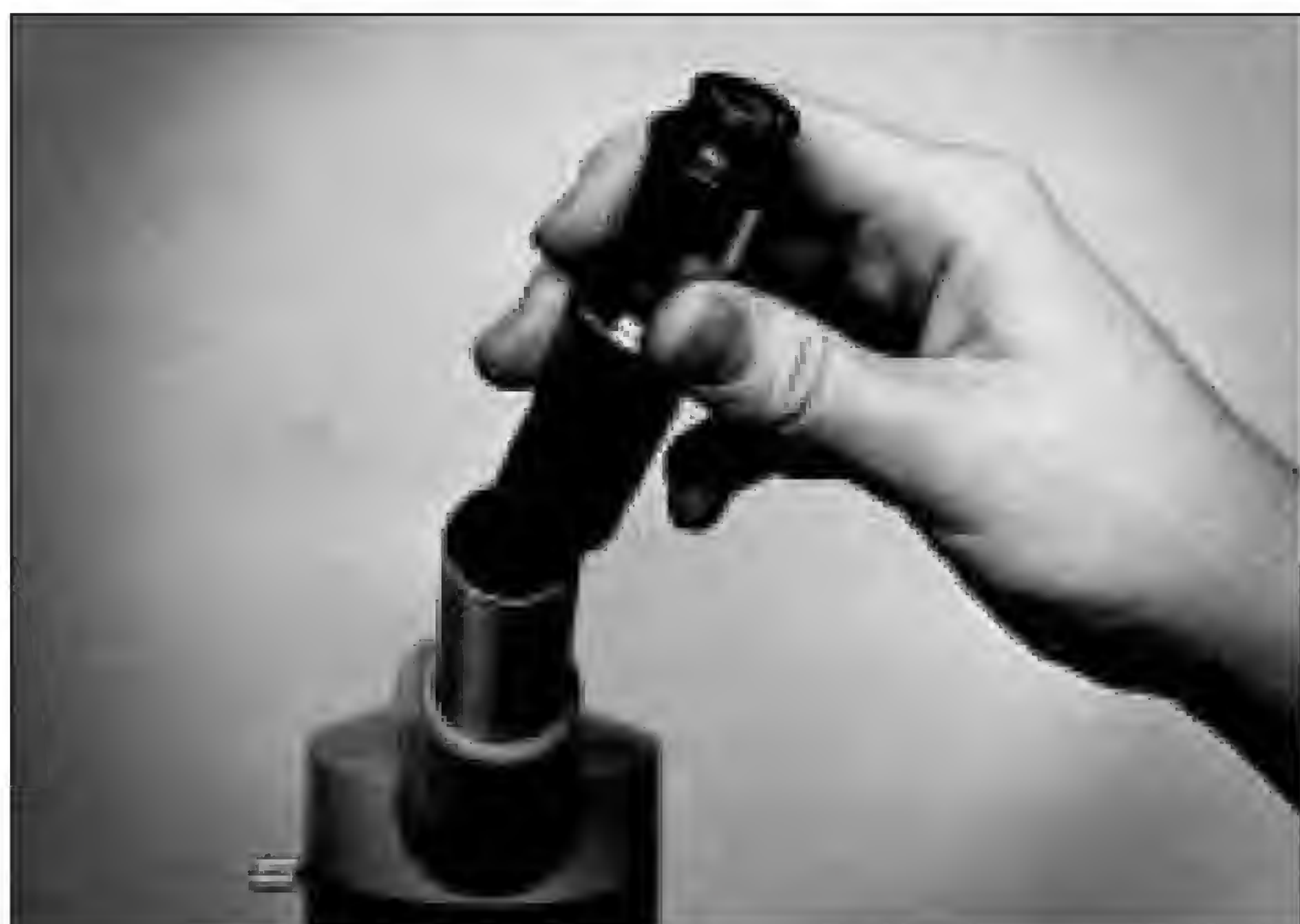
Figure 3.7 If the ocular of a phase-contrast microscope is replaced with a centering telescope, the orientation of the phase ring and annular ring can be viewed.
