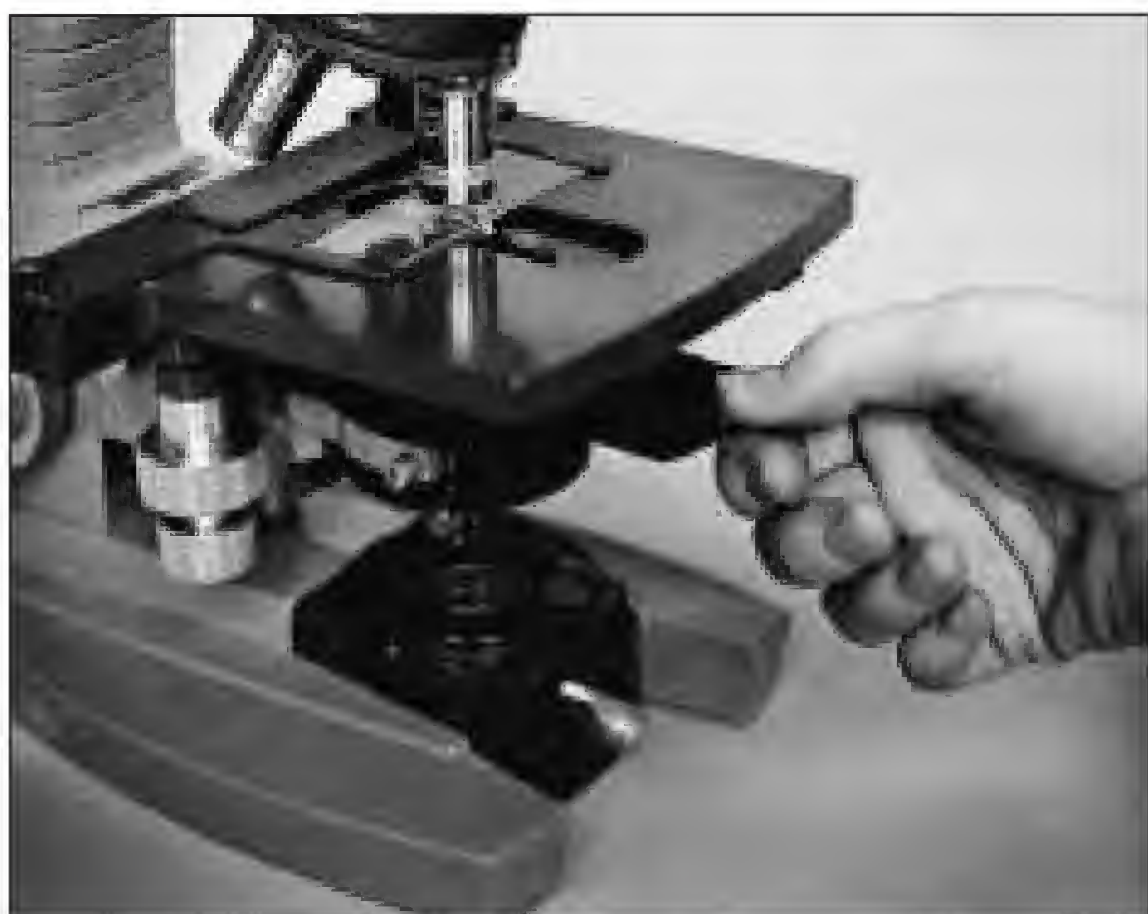
Figure 3.9 The annular stop on this American Optical microscope has the annular stop located on a slideway. When pushed in, the annular stop is in position.
