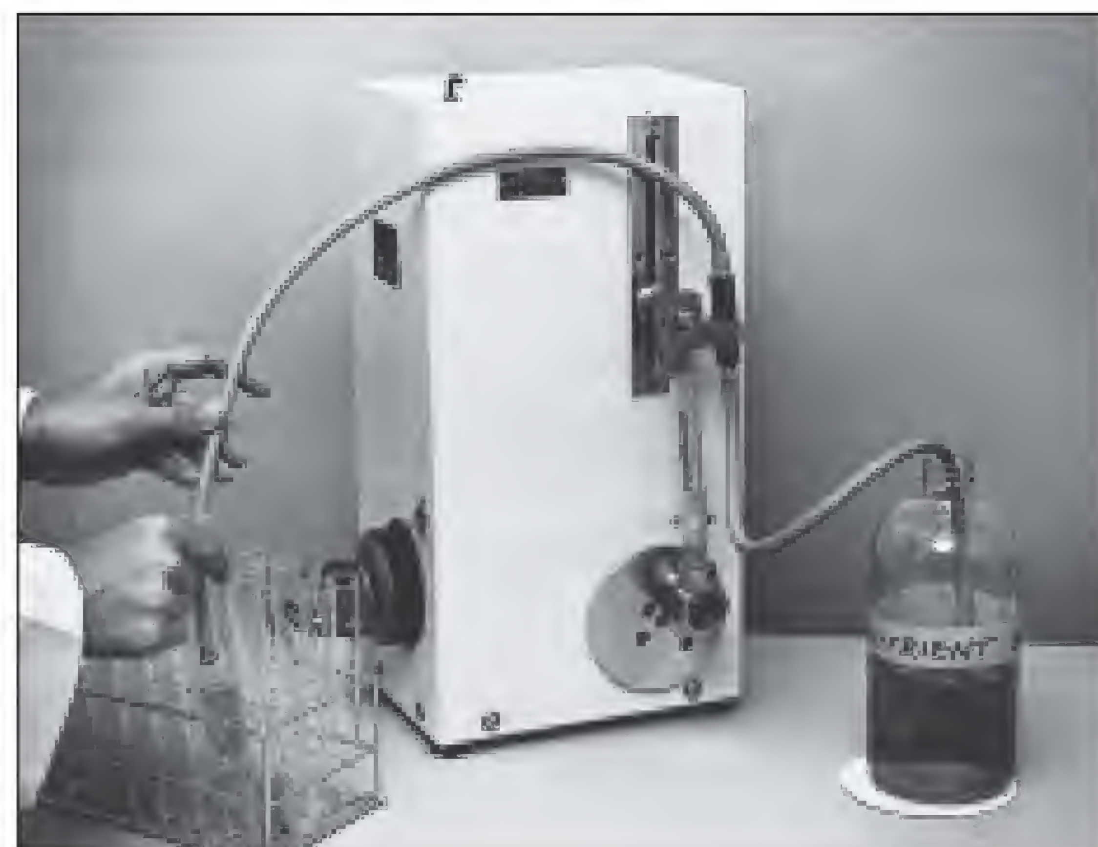
Figure 20.6 An automatic pipetting machine will deliver precise amounts of media at a controlled rate.
