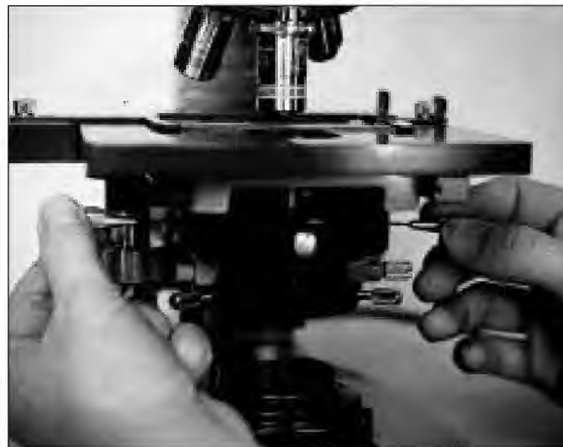
Figure 3.5 Alignment of the annulus diaphragm and phase ring is accomplished with a pair of Allen-type screwdrivers on this American Optical microscope.
