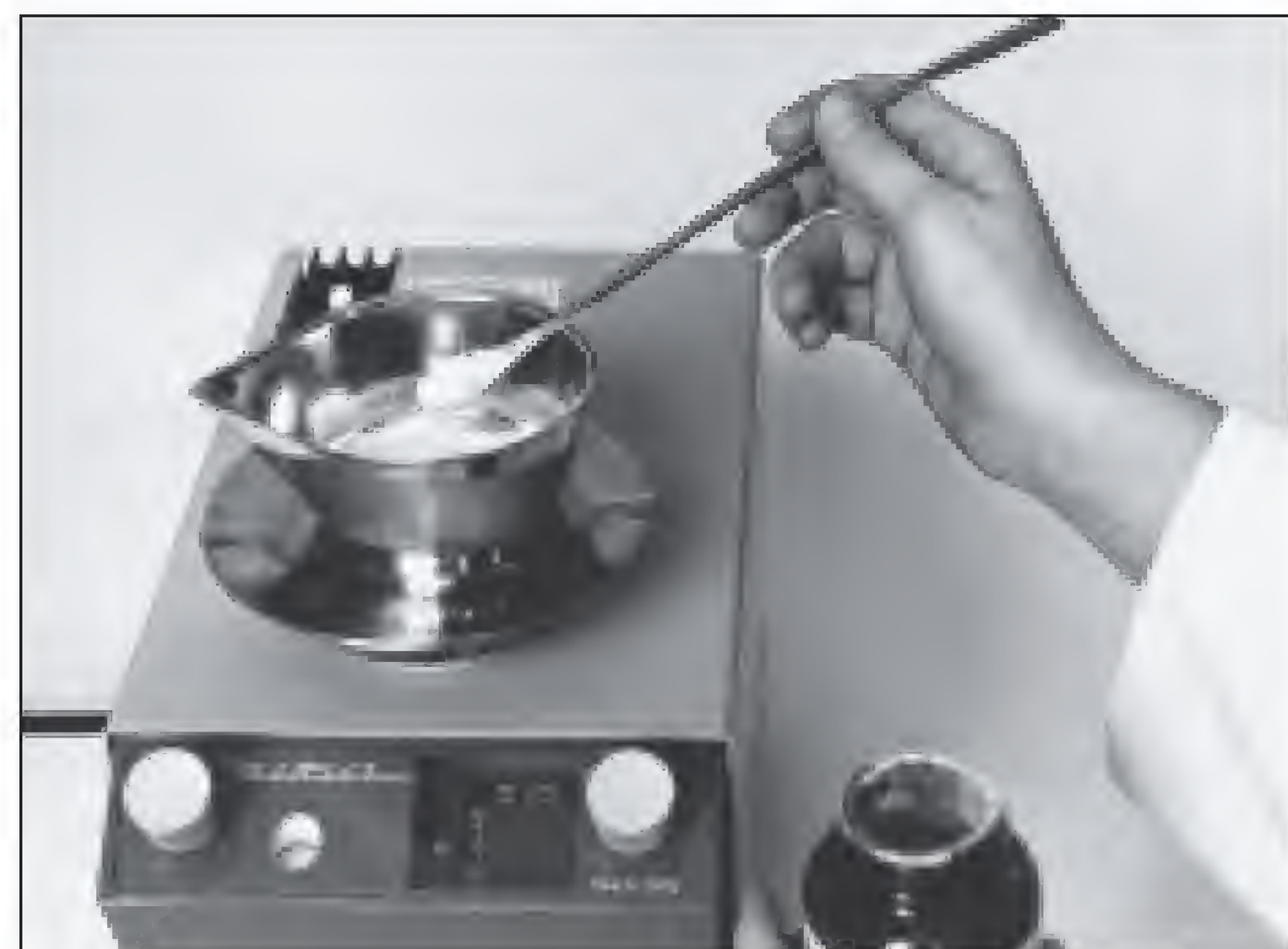
Figure 20.2 Correct amount of dehydrated medium is weighed on balance.
