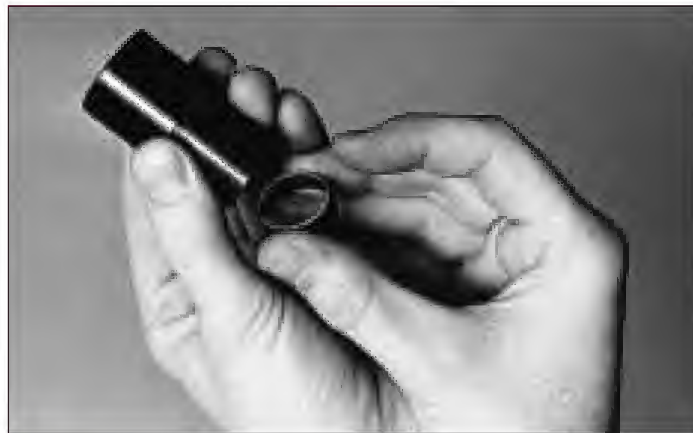
Figure 5.1 Ocular micrometer with retaining ring is inserted into base of eyepiece.
