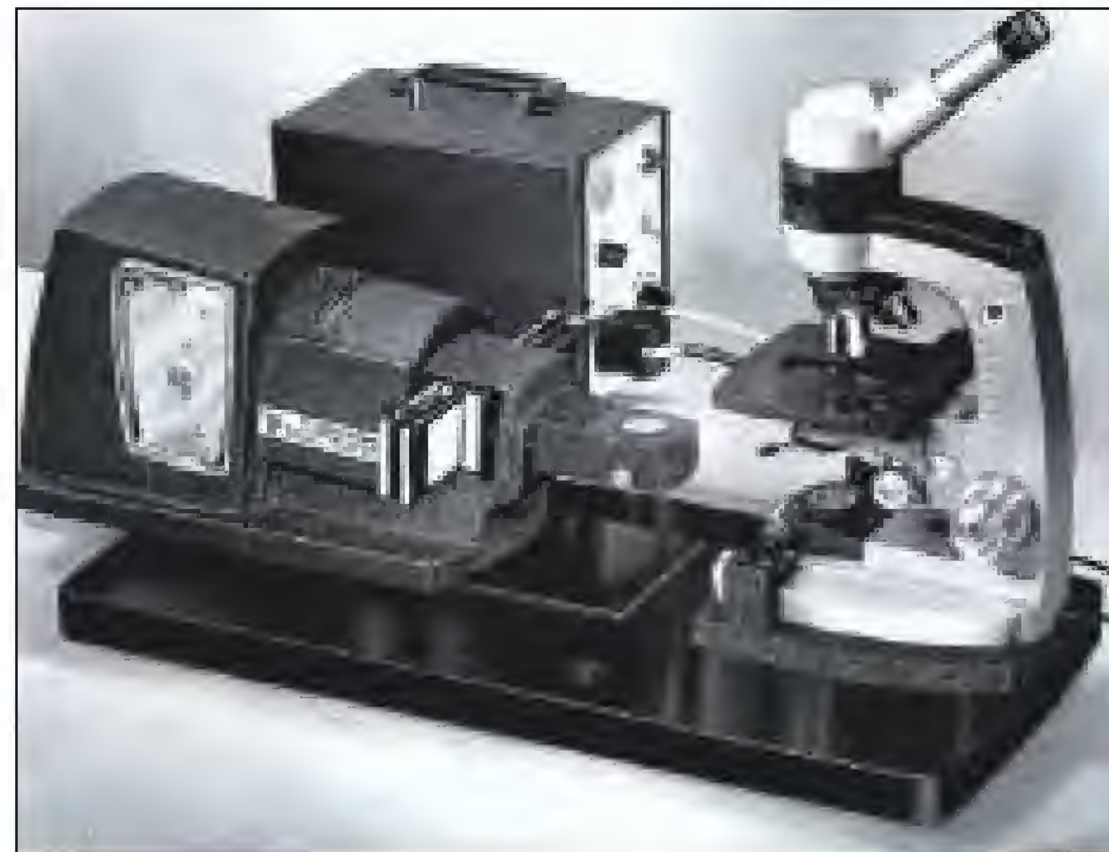
Figure 4.1 An early model American Optical fluorescence illuminator ( Fluorolume ) that could be adapted to an ordinary darkfield microscope.
