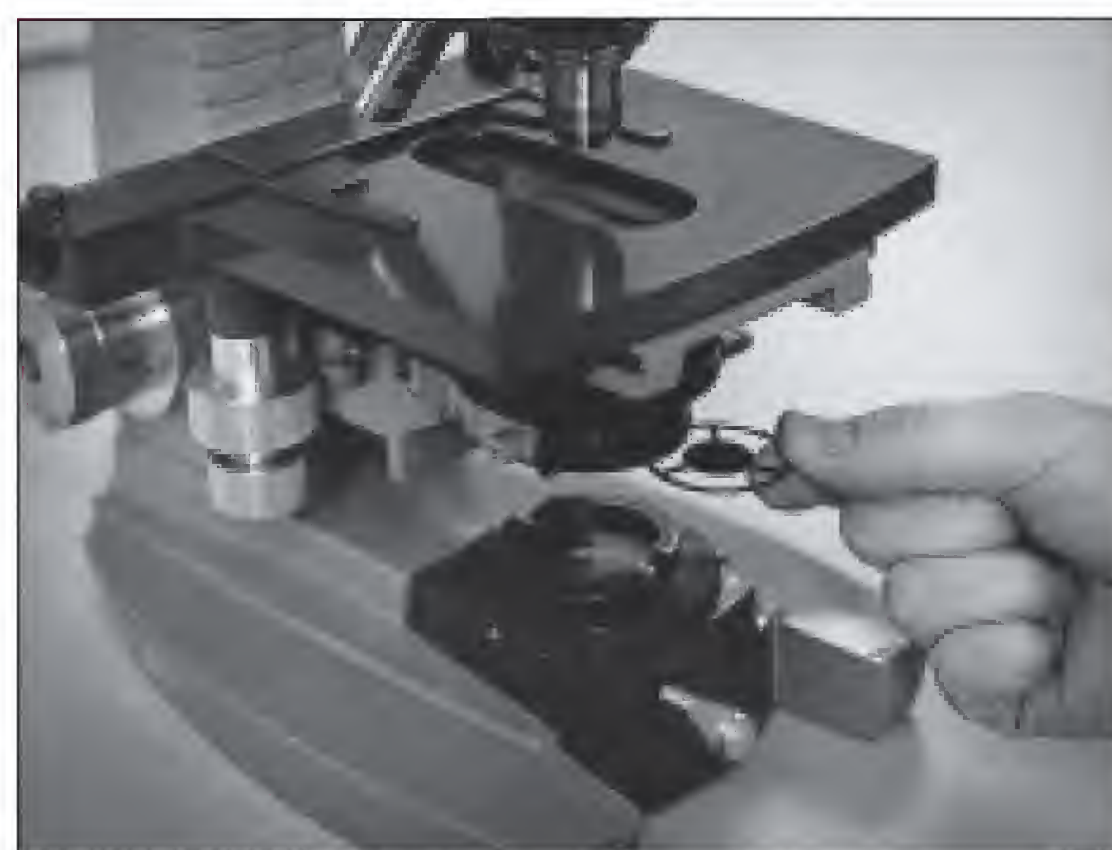
Figure 2.2 The insertion of a star diaphragm into the filter slot of the condenser will produce a dark field suitable for low magnifications.
