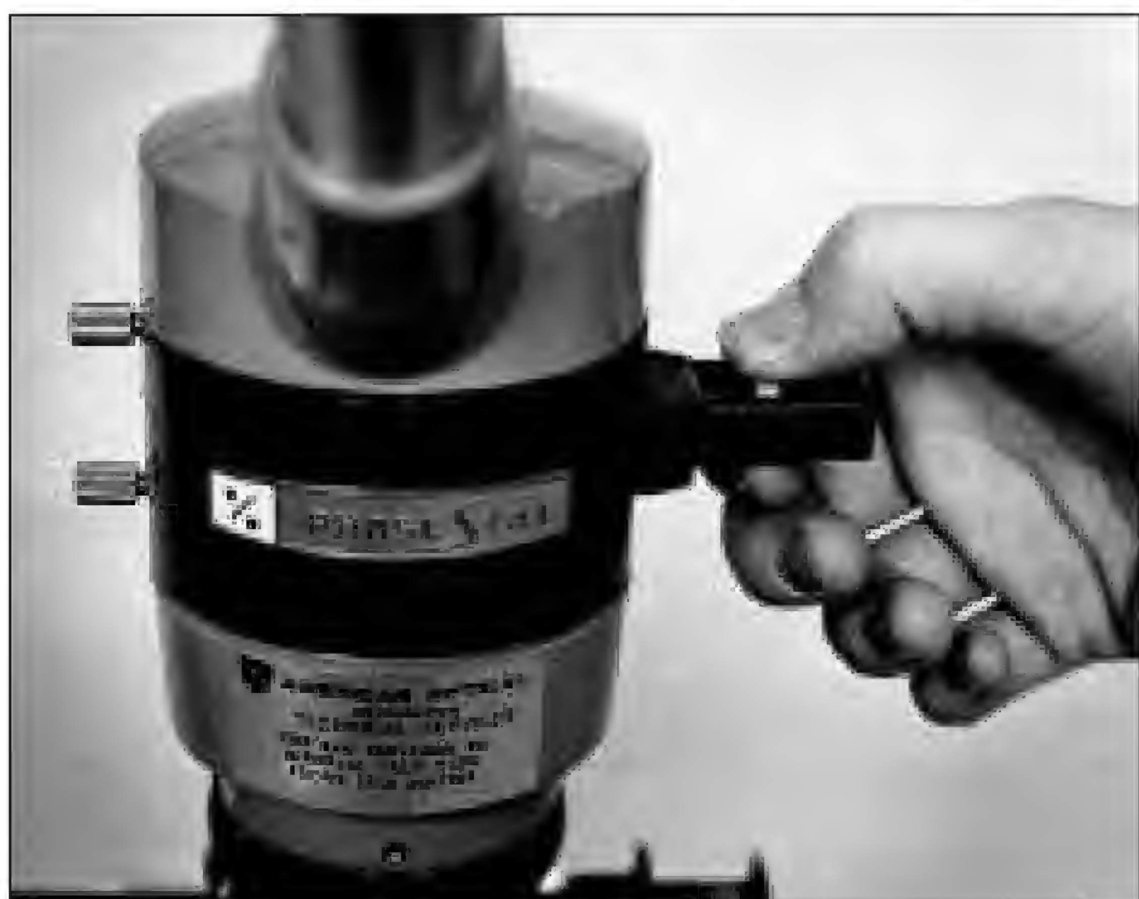
Figure 3.8 Some microscopes have an aperture viewing unit that can be used instead of a centering telescope for observing the orientation of the phase ring and annular ring.
