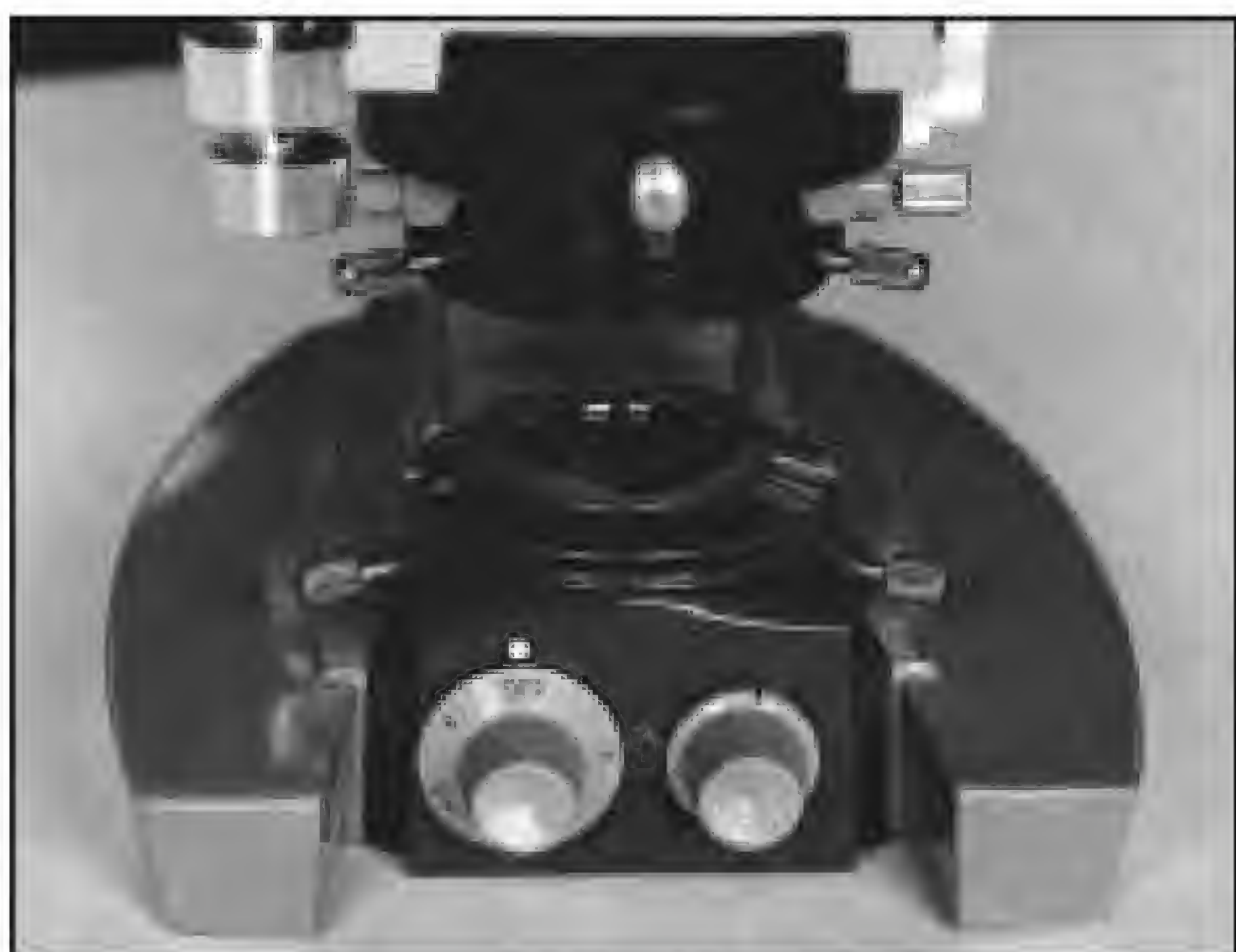
Figure 1.4 On this microscope, the left knob controls voltage. The other knob is used for moving a neutral density filter into position.
