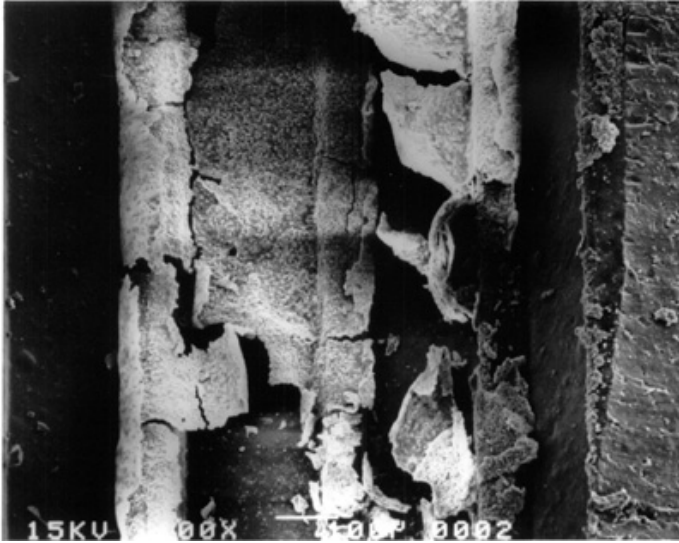
Figure 3. SEM image of ureteral stent recovered from a patient. The stent was opened longitudinally to show the extent of encrustation which was almost sufficient to block the flow of urine.
