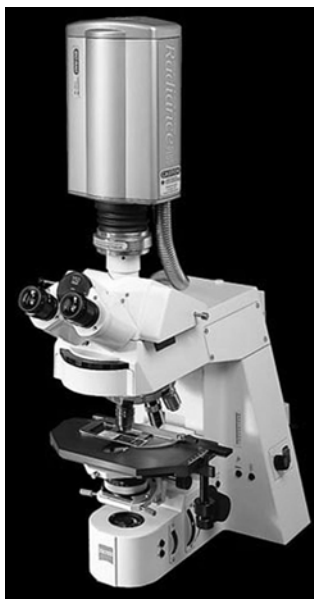
Figure 6. A recent model of CLSM system, Radiance Plus (Courtesy Bio-Rad, Hercules, CA).
