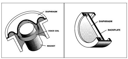
Cutaway view of dynamic (left) and condenser microphone cartridges
