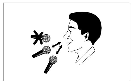
Illustration: Ideally, a handheld microphone should be positioned six to twelve inches from the user's mouth, at an angle of 45 degrees or less. This usually avoids air currents that result in "popping" sounds when the consonants "P" or "T" are pronounced.
