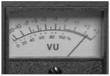
Average VU meter reading if level is set too high; may result in signal overload distortion
