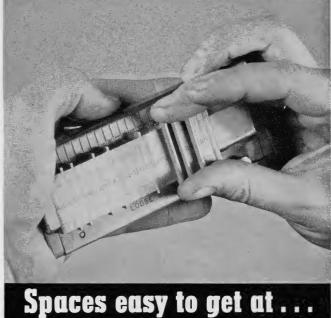
In the composition of single types, it is the spaces which have to be handled most frequently in setting and justifying a line. Yet these spaces are far below the face of the line and are the hardest units in the line to get at.
