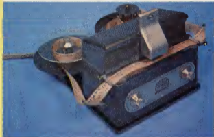
Because there is no sprocket feed in the reader, unevenly perforated tape can be used without difficulty. Mechanical readers require 10 signals per inch, but the AutoSetter system will accept wide variations from the former exact tape standards.
