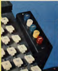
These five buttons control all tape operations. From here the tape may be stopped, started or reversed. For manual operation, there are also buttons for raising the elevator, and for shifting to upper or lower rail positions.
