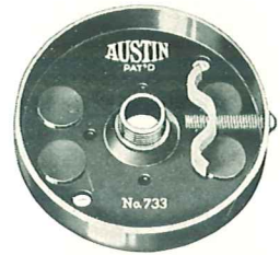
No. 733 \frac{1}{2} " Deep, 3\frac{1}{2} " Diameter, \frac{3}{8} " Fixture Stud; Four \frac{5}{8} " K. O. One Clamp
