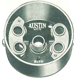
No. 731 1\frac{1}{2} " Deep, 3\frac{1}{2} " Diameter, \frac{3}{8} " Fixture Stud; Four \frac{5}{8} " K. O. with Bushing Plates
