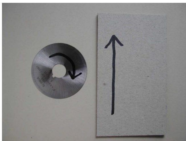
Fig. 6- Every board slotting machine should be operated in this direction when cutting.
