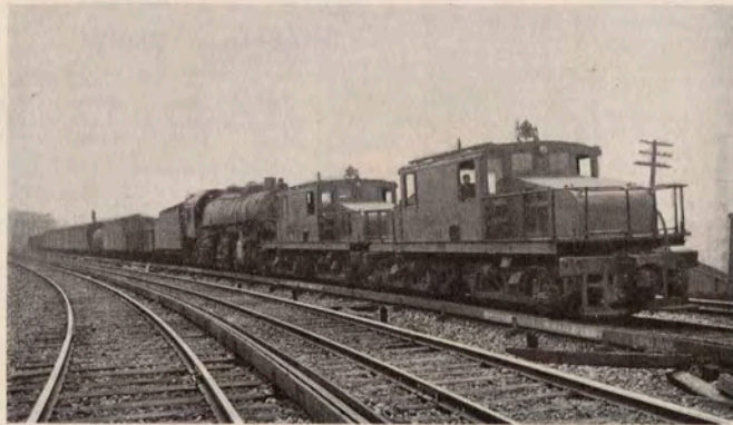
Fig. 7. Two 100-ton Freight and Passenger Locomotives, Type OE-1 and OE-2, each equipped with four GE-209 Motors hauling freight train
