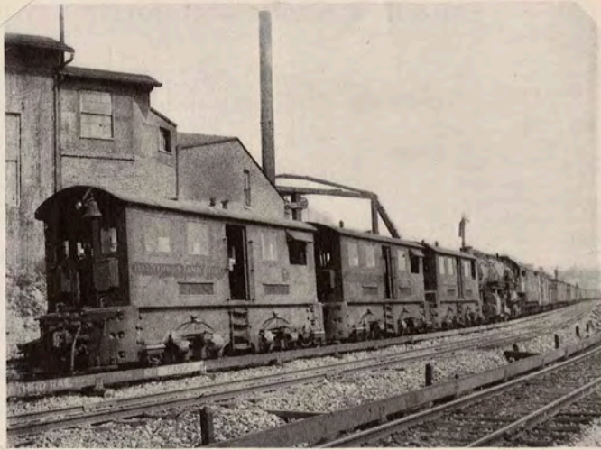
Fig. 5. Three 80-ton Freight Locomotives, Type LE-1 and LE-2, each equipped with four GE-65 Motors hauling freight train
