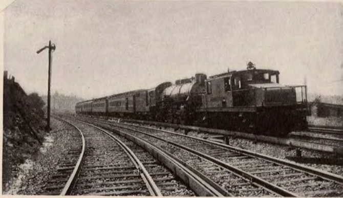
Fig. 6. One 100-ton Freight and Passenger Locomotive, Type OE-1 and OE-2, equipped with four GE-209 Motors hauling passenger train
