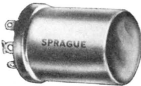
FIG. 44-E.—Sprague electrolytic capacitors. At the upper left is a filter capacitor mounted in a paper box; at the upper right, a by-pass capacitor; at the bottom are etched foil capacitors with self-mounting features.
