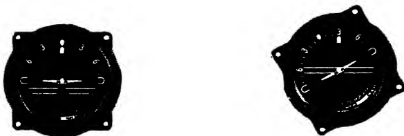
Fig. III. 41. Pre-war civil type. Sperry artificial horizon, dial indication. (Left) Climbing. (Right) Left bank. The latest type has a single line horizon with bank scale at the bottom of the dial.
