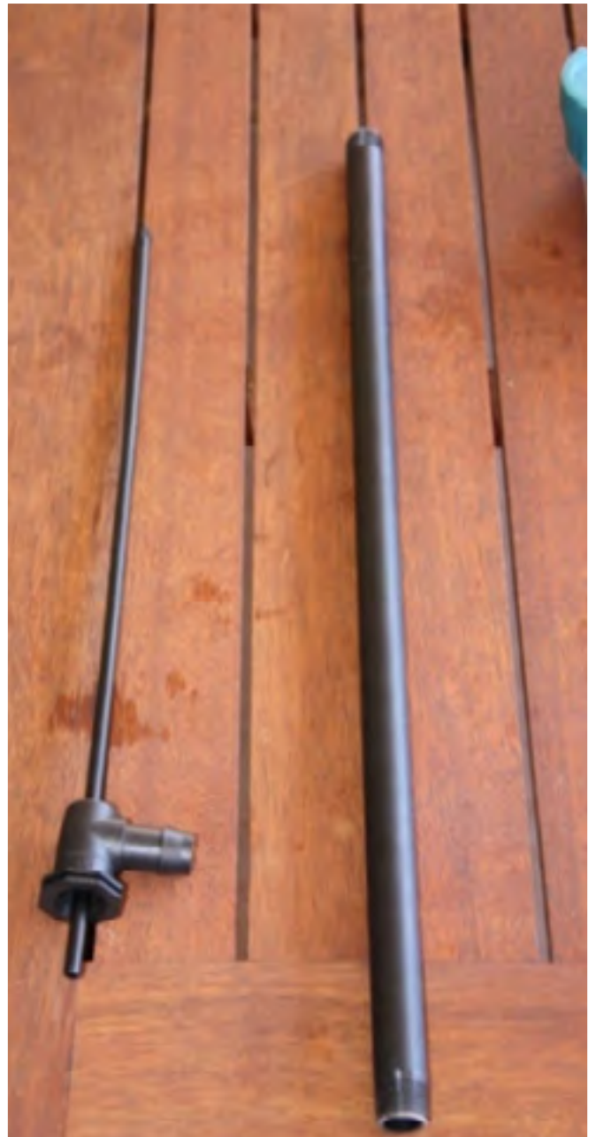
Venturi, all made from reticulation parts
