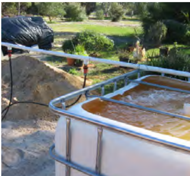
Tank and polypipe returns
