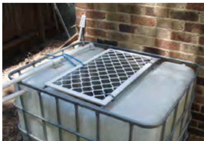
Security screen stops unwanted visitors and debris entering the container and can be opened to gain access for fish harvest
