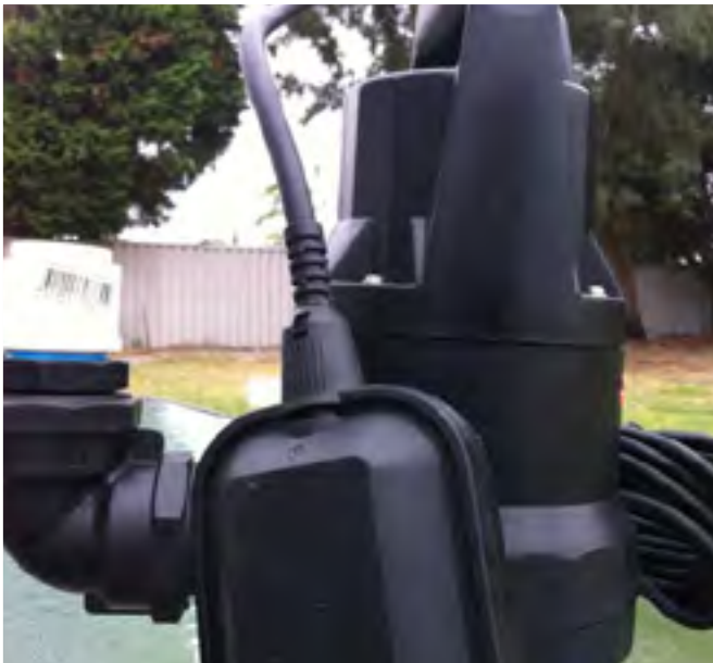
Pump with float switch
