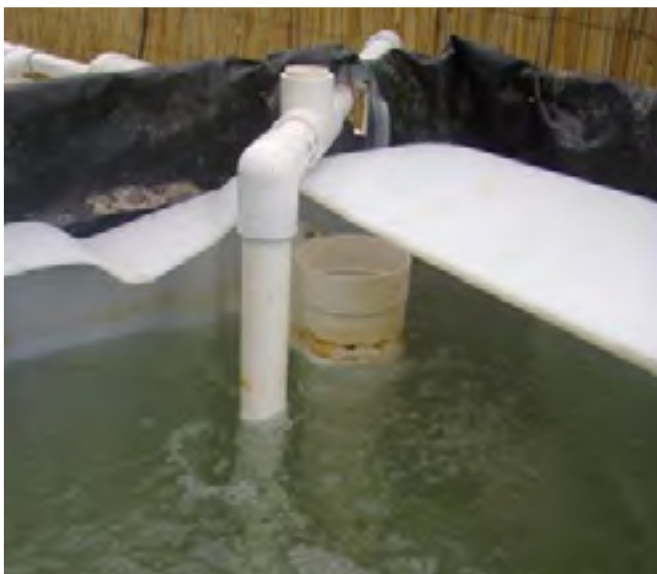
Here we can see the bubbles from the venturi sucking air into the water stream. Also the 90mm Solids lift overflow in the background
