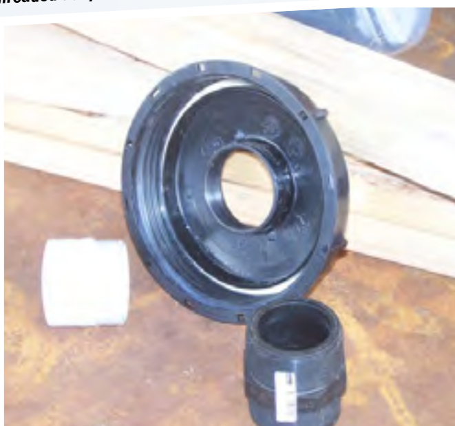
2 inch thread on lid makes for easy adaption
