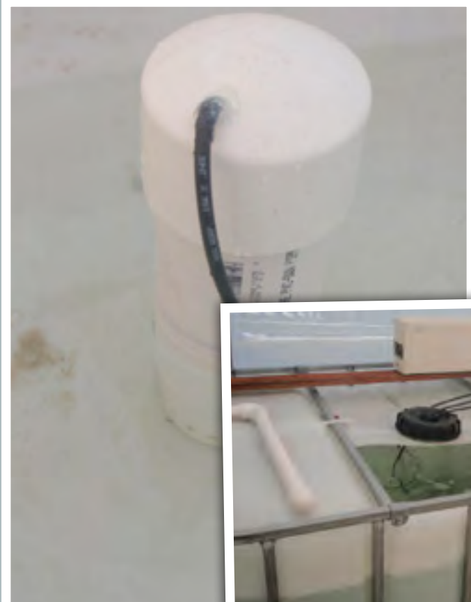
Two different siphons were tried, one bell siphon with a breather hose
