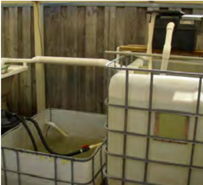
Extra external filters have been added to the system over time
