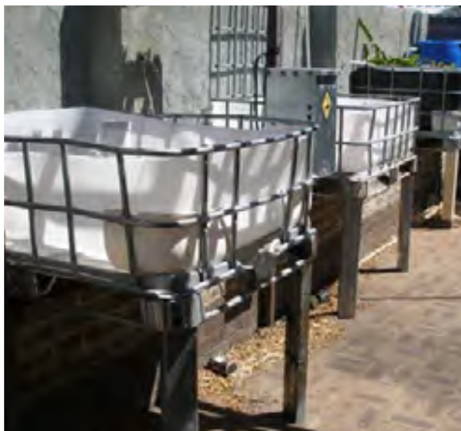
Square patio tubing supports the front of the growbeds
