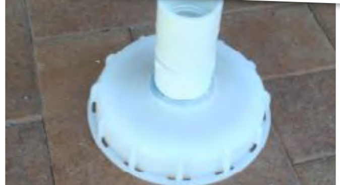
Fittings installed in the lid of the IBC
