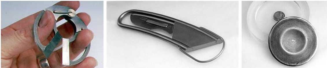
figure 4: knives made by Horne (left to right) little snips in cast stainless steel, folding scalpel in cast stainless steel with disposable blade, disc knife in Damascus steel with silicon/magnet holder
