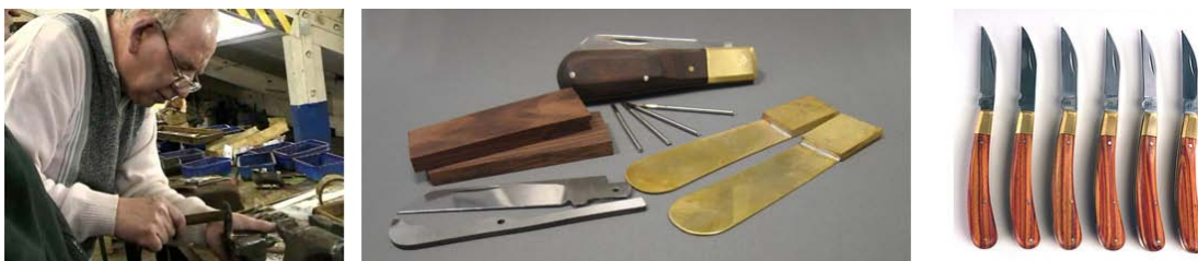
figure 6: (left to right) Trevor Ablett, parts of a traditional folding knife, set of "Ettrick" folding knives made by Horne under Ablett's guidance
