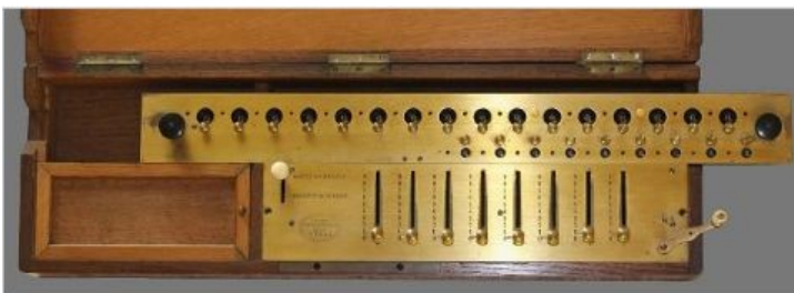
Front panel of a Thomas arithmometer with its movable result carriage
