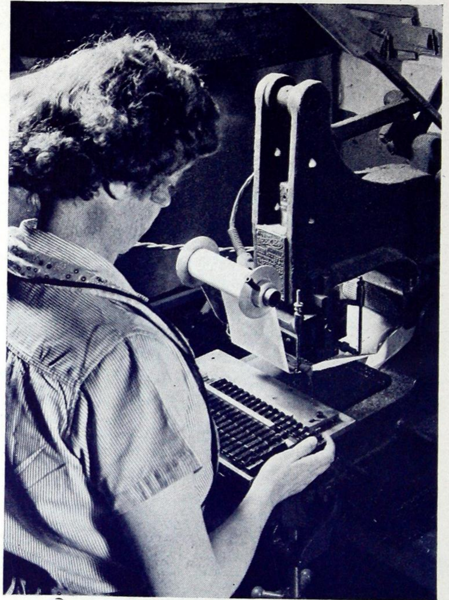
This is a roll automatic stamping device for labeling and numbering molded sections of either thermoplastic or thermosetting materials.
