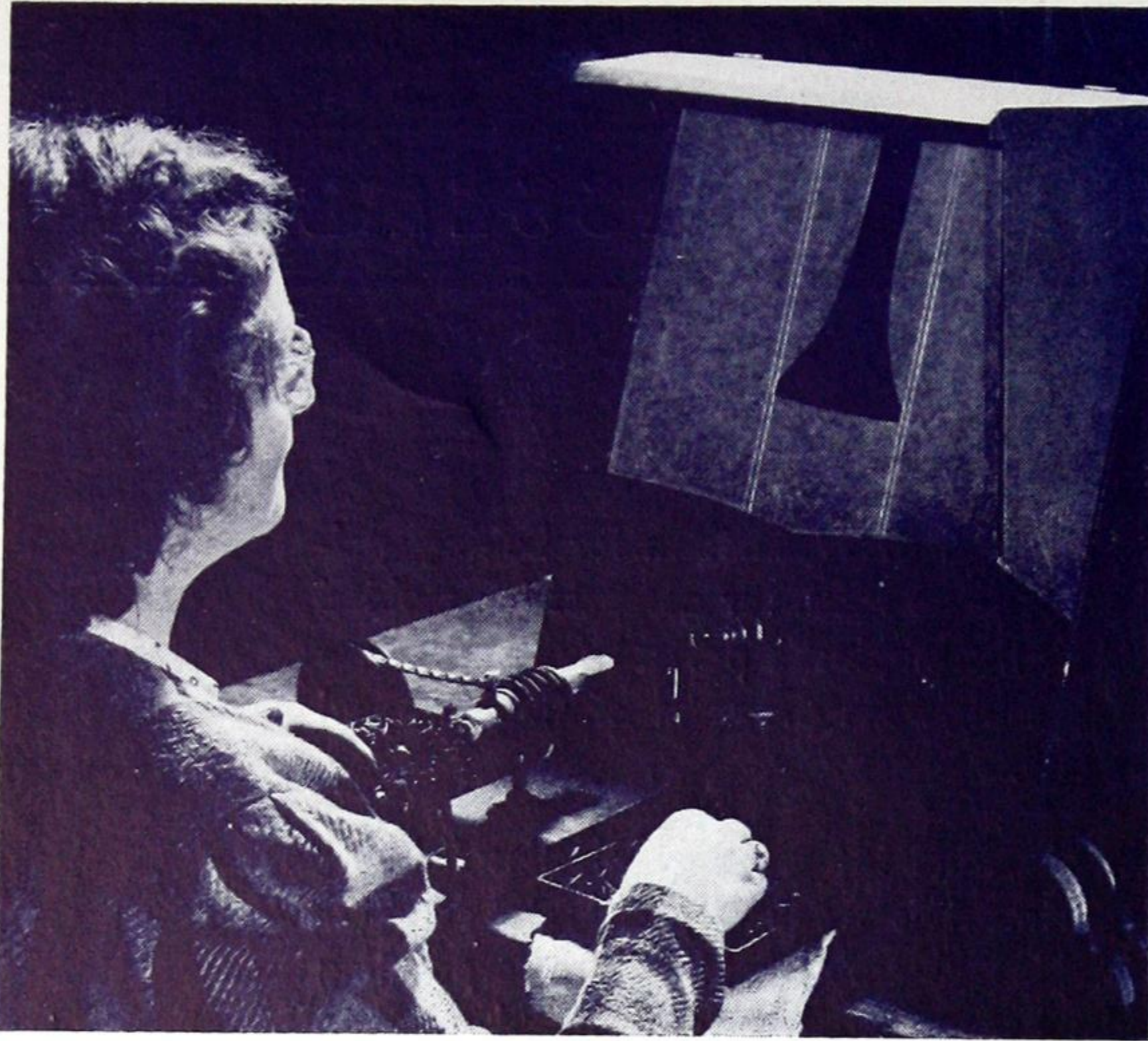
This illustration shows the Shadowgraph which measures the concentricity of the very tiny firing pins. The Shadowgraph enlarges the pin 30 times and any section extending beyond the white line means that the pin must be rejected.
