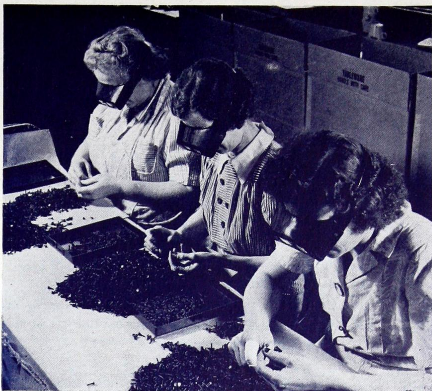
In addition to Shadowgraph inspection for perfect concentricity, each firing pin undergoes rigid inspection. Porosity or any imperfection is quickly detected.
