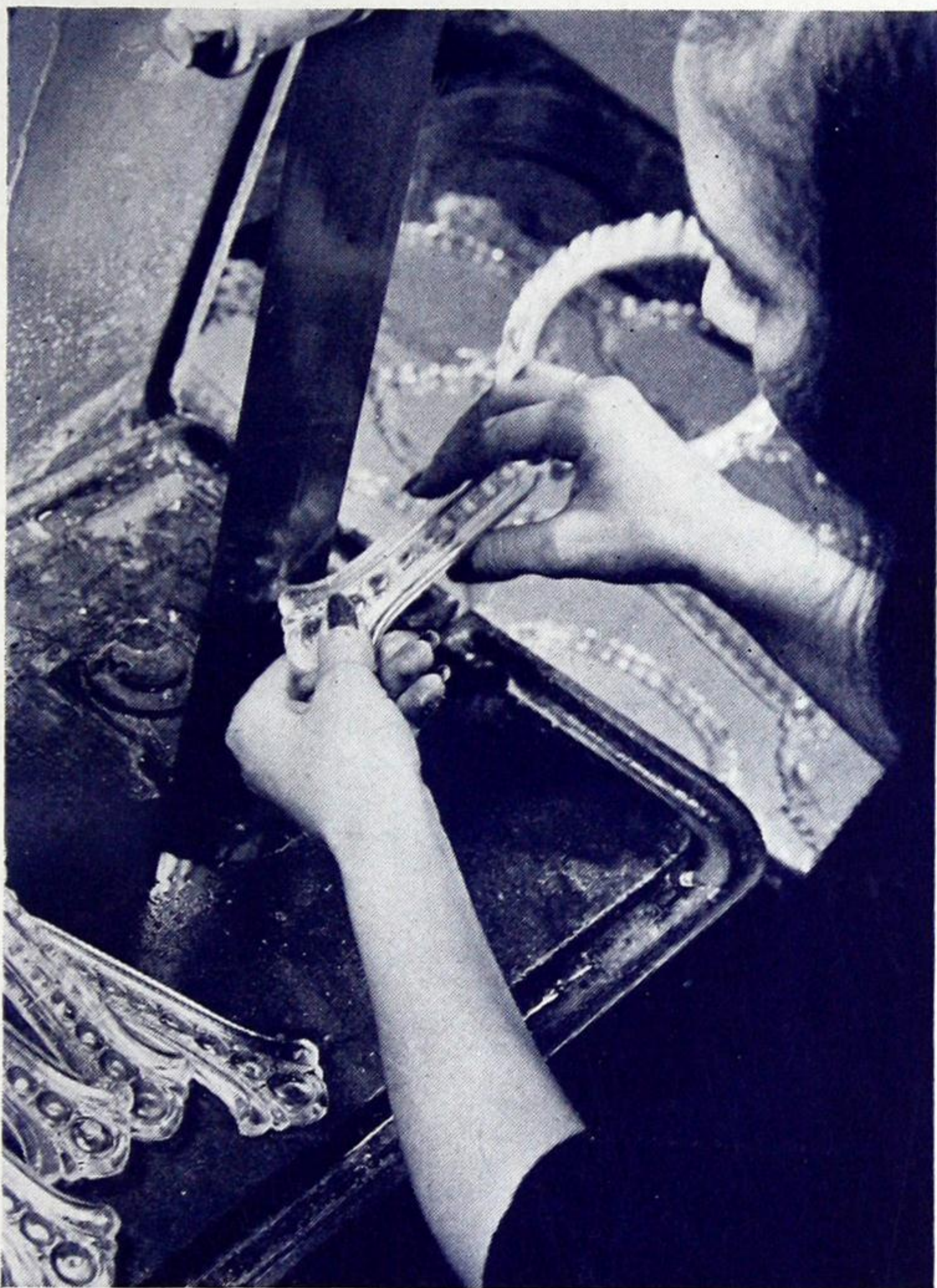
Here the gate is being removed and the spot polished on Lucite mirror and brush handles.
