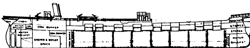
The Charlois (designed by Messrs. Flannery & Blakiston), of which it was said that her structure, sub-divided by bulkheads into compartments of moderate size, formed the necessary receptacle for carrying the oil. She was an innovation and an improvement on the system of building separate tanks into the ship.
