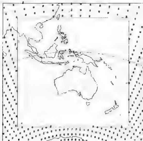
Fig. 5 Schematic showing the nesting of the LAM grid within the CSIRO GCM grid over Australia.
